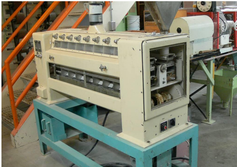
Fig.2.13 MIAG laboratory purifier (MIAG, Braunschweig, Germany)
