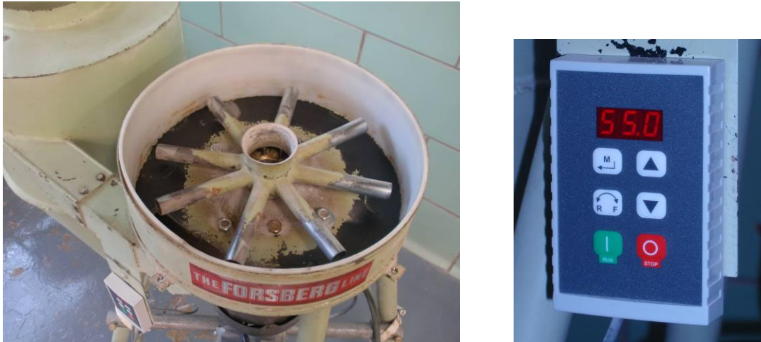
Fig.2.5 Centrifugal device and remote control of Impact Forsberg machine
