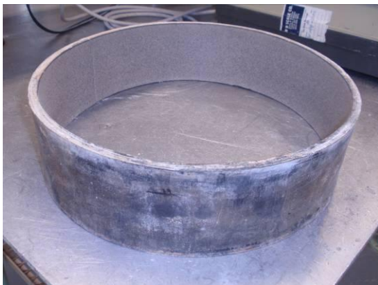
Fig.2.4 Rubber and Plastic Inner Rings for Impact Forsberg Machine
