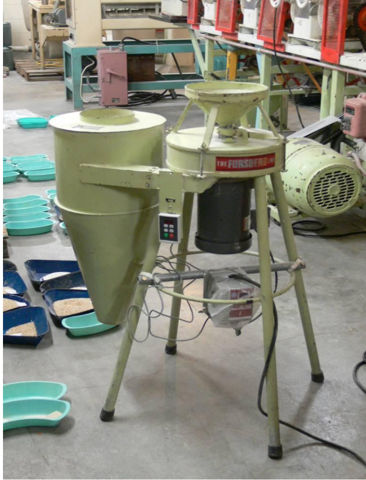
Fig.2.3 Impact Forsberg machine (Forsberg's, Inc., Thief River Falls, Minnesota)
