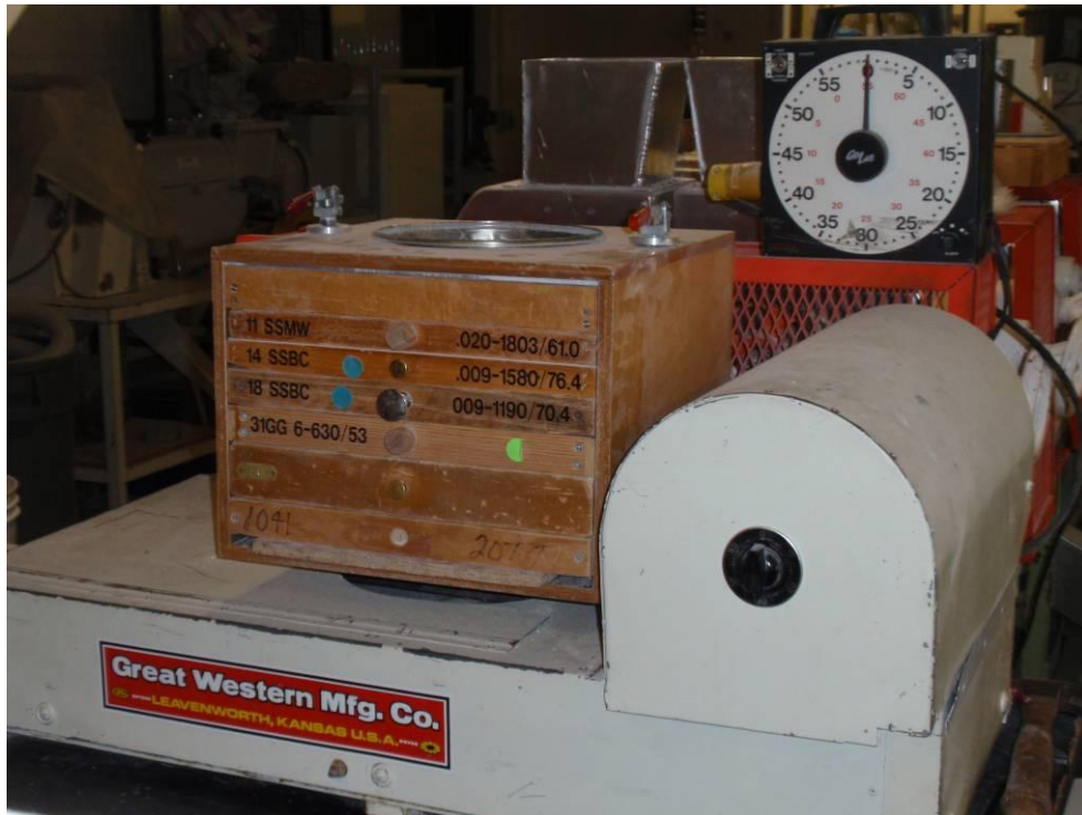
Fig.2.6 Laboratory Sifter (Great Western Manufacturing, Inc., Leavenworth, KS)
