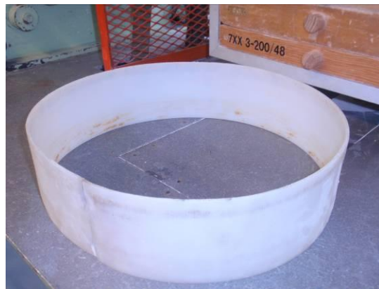
Fig.2.4 Rubber and Plastic Inner Rings for Impact Forsberg Machine
