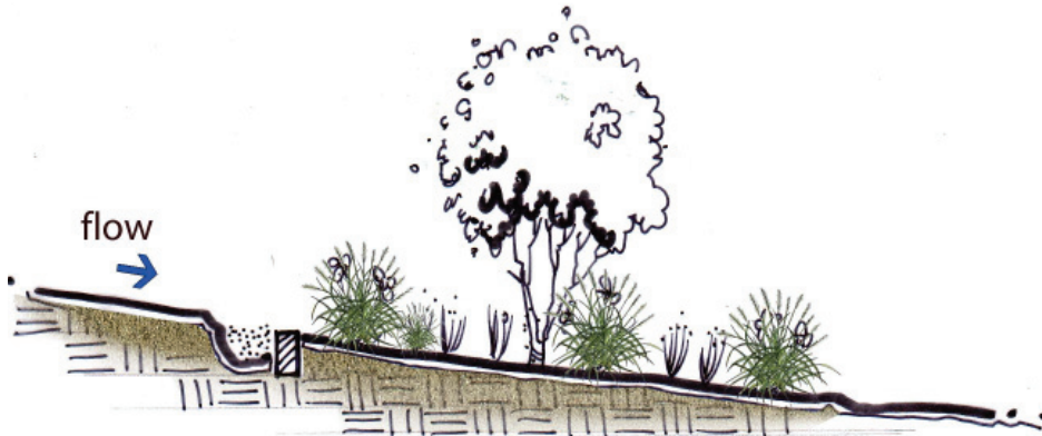
Figure 7.6 Filter Strip (Cody Peratt 2008, Adapted From Portland Bureau of Environmental Services 2008 Stormwater Management Manual)
