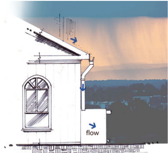
Figure 7.11 Rainwater Harvesting (Cody Peratt 2008, Adapted From Portland Bureau of Environmental Services 2008 Stormwater Management Manual)
