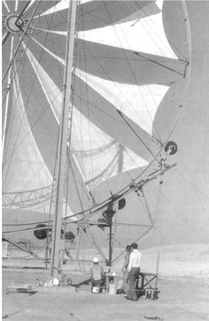
Figure 13. Windjammer turbine being tested in California. Photograph copyright 2002 Gordon G. Brittan Jr. from Architectural and Environmental Phenomenology Newsletter , 13 (2).
