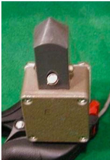
Figure 1.11 Photocell Array From WattSun Solar Tracker
