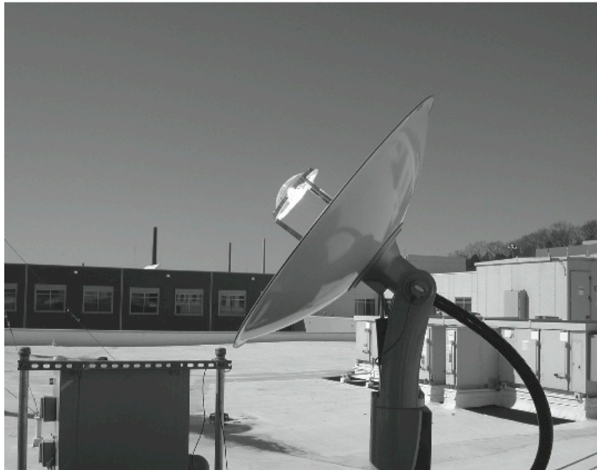
Figure 1.7 ORNL Parabolic Reflecting Collector
