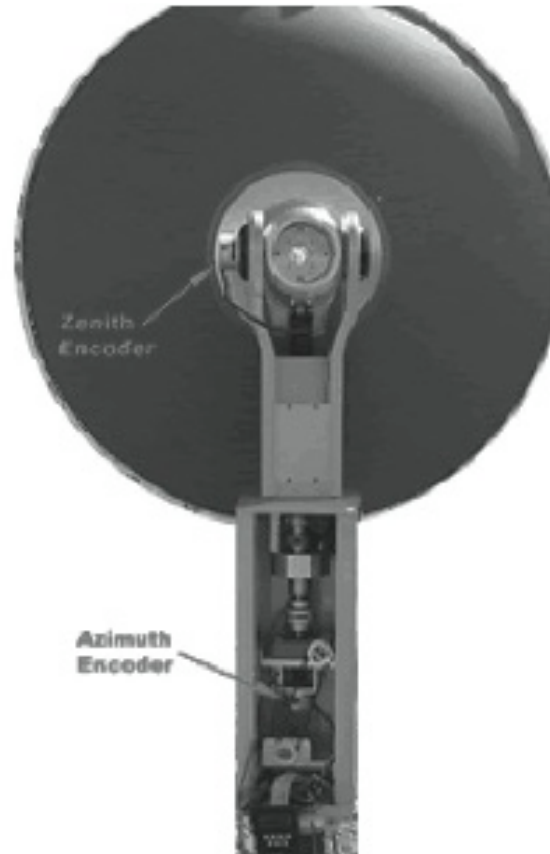
Figure 1.12 Astronomical Tracking System on ORNL Parabolic Solar Collector
