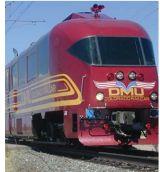
Figure 4.1 - DMU Commuter Rail Car. Commuter rail trains use DMU cars like this train in Colorado. Source: FasTracks Regional Transportation District of Denver.
