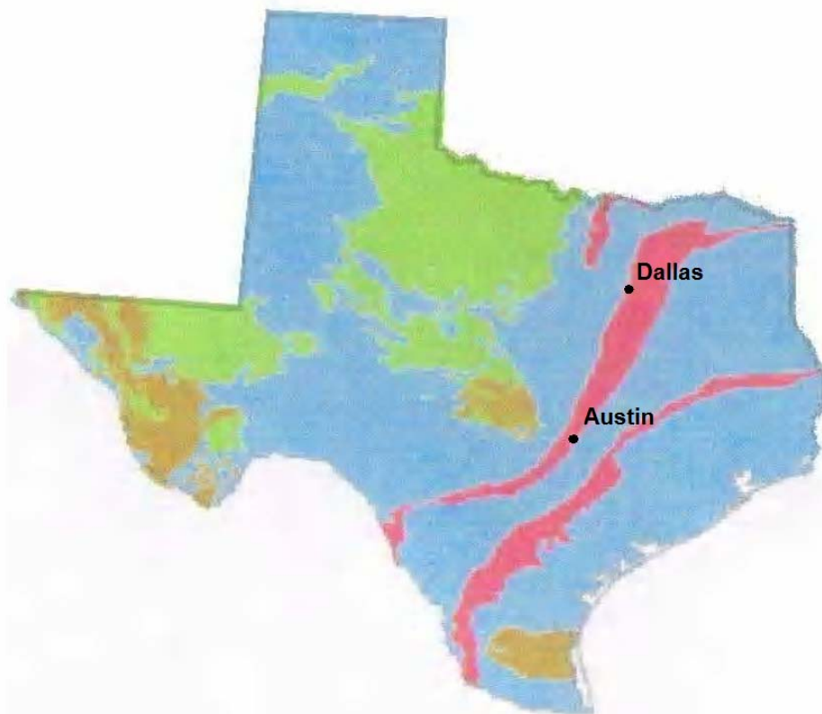
Figure 4-2. Expansive Soils in Texas
