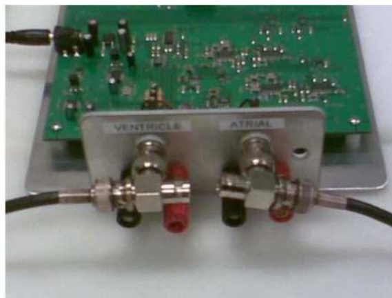
Figure5.2 : Connecting the pacing leads to Atrial and Ventricle Ports ( http://www.cas.mcmaster.ca/~lawford/pacemaker/user_guide.pdf )
