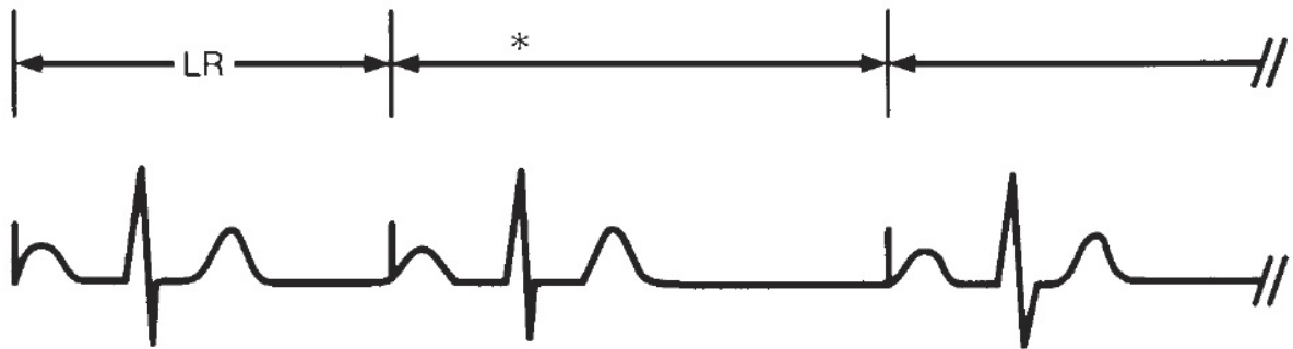
Figure4.21 : Far-Filed Sensing in AAI mode
