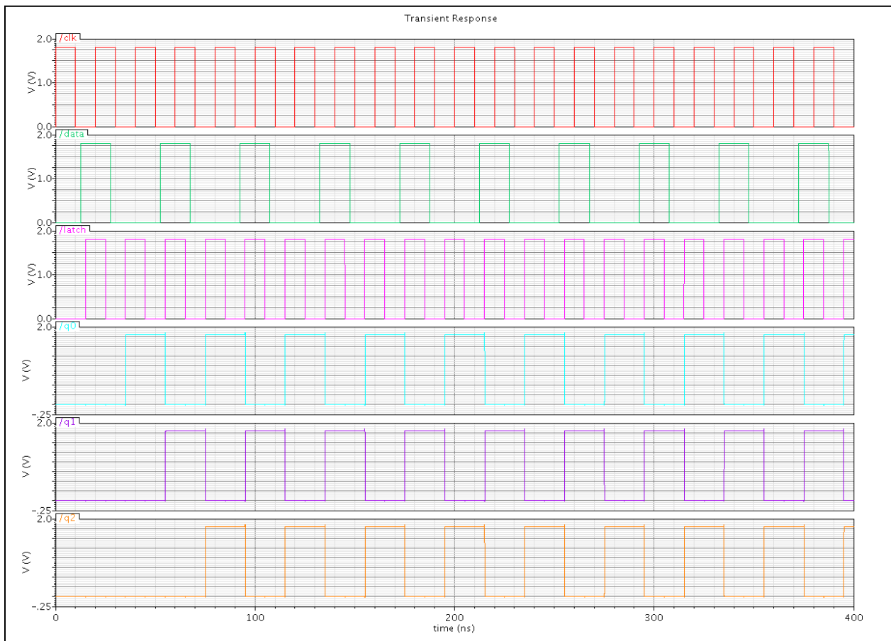
Figure A.6 – Simulation Output for Serial to Parallel Register
