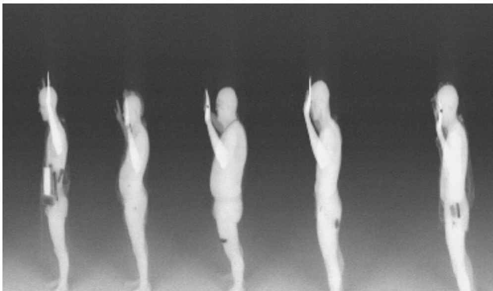
Figure 2-2: Standoff X-ray detection showing hidden explosives and other items on personnel. Images were taken from a van moving at 0.3 to 6 miles per hour using X-ray backscattering in “drive-by” mode. The mock suicide vest contained simulated C4 explosives and pipe bombs. Both the explosives and the pipe bombs are easy to see and are distinguishable from normal objects under clothing (NRC, 2004).
