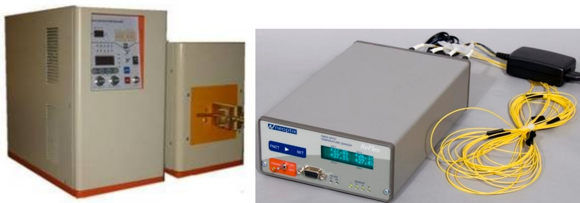
Figure 6.4 Induction heater (left) and fiber optic temperature probe (right) for magnetic hyperthermia experiment.
