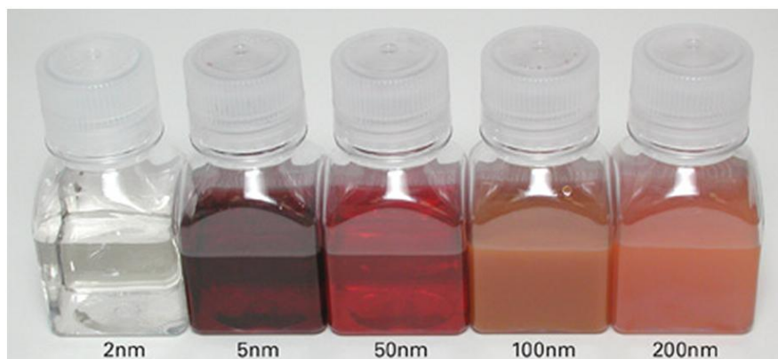
Figure 1.8 Nanometersized monodispersed gold colloids of different sizes in water, with trace amounts of citrate, tannic acid and potassium carbonate ( http://www.tedpella.com/gold_html/goldsols.htm ).
