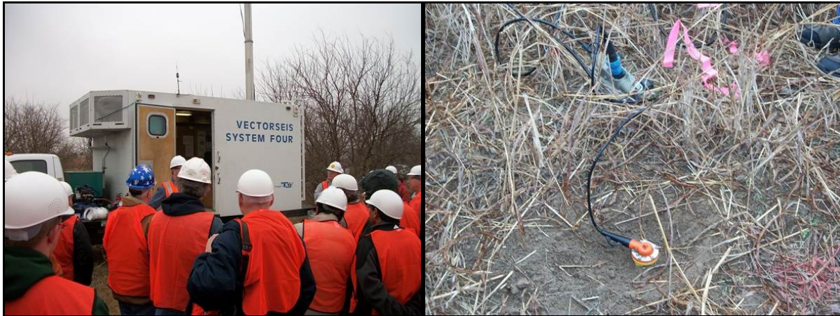
Figure 13 Shows the Paragon Geophysical Services recording station. Figure 14 Shows the single 3C Digital geophone planted in the ground ready for listening.
