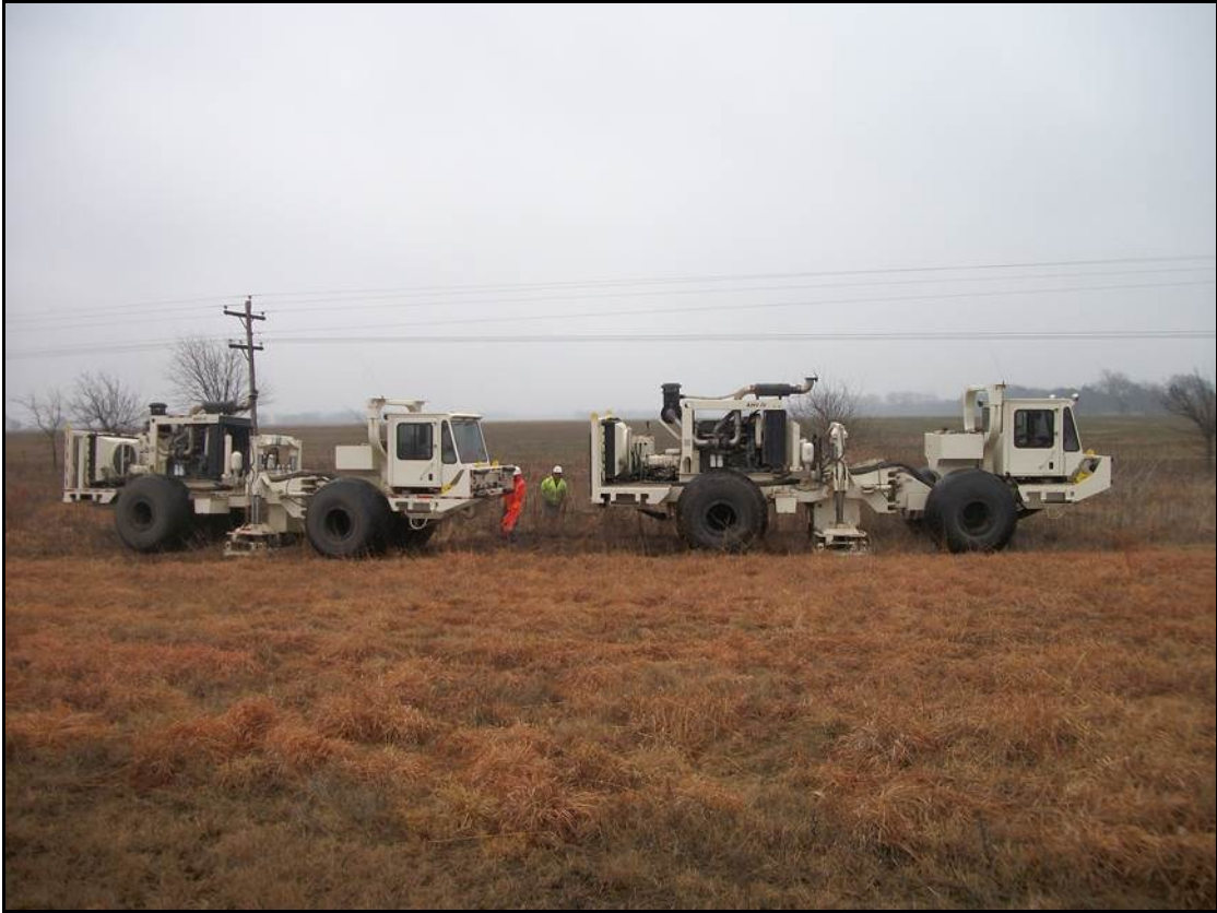
Figure 15 Shows the two vibroseis sources used to acquire the seismic data.
