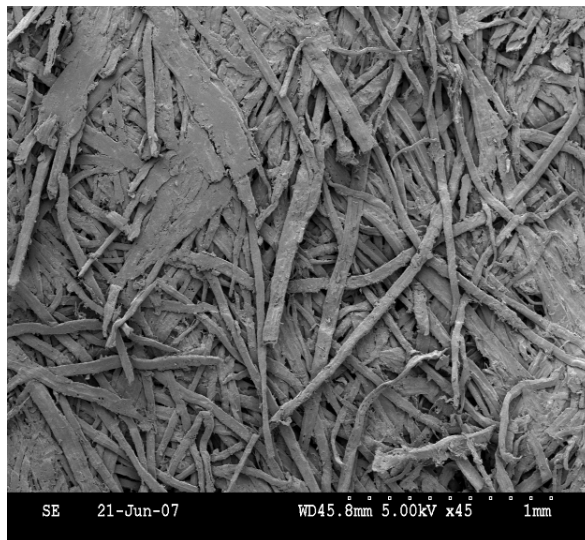
Figure 2-3 Scanning Electron Micrographs of the Fractured Surface of Wood Fiberboards.
