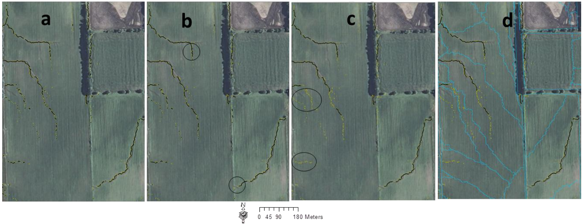
Figure 4.6 Steps in deriving the length of ephemeral gullies (EGs): (a) EG raster converted to polyline, (b) polylines snapped, (c) length of EGs calculated and smaller lengths <10 m deleted, and (d) EGs were given unique id. Black polylines represent EGs, and blue polygons represent EG catchments.
