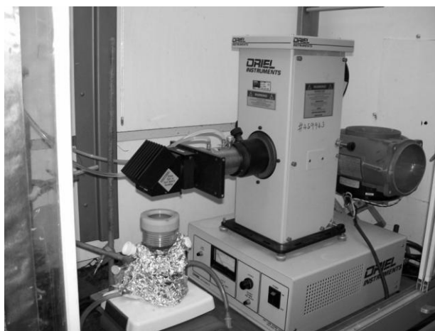
Figure 1-3 Shown above is the glass reaction vessel with the quart glass window top and the Oriel 1000W high pressure Hg lamp used to produce visible light.
