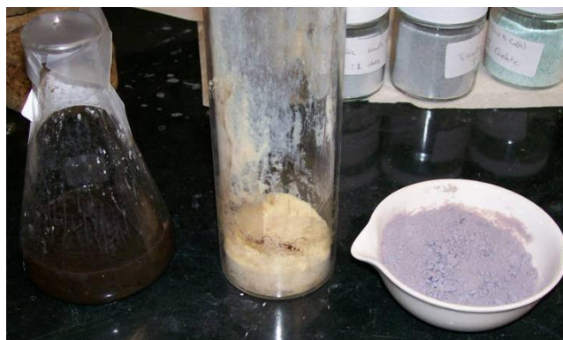
Figure 1-13 Shown above left to right is the wet gel, aerogel after supercritical drying and finally the calcined aerogel (finished product).
