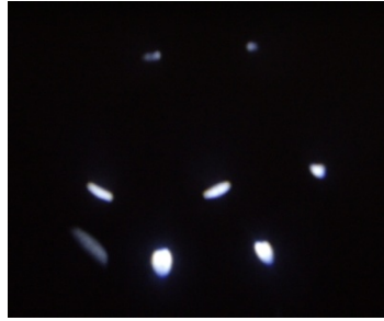
Figure 4.7 Aberrated grid pattern
