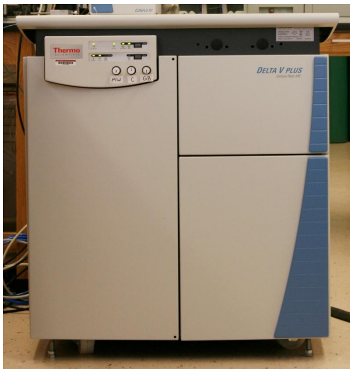
Figure 5. The Delta V + isotope ratio mass spectrometer (IRMS).
