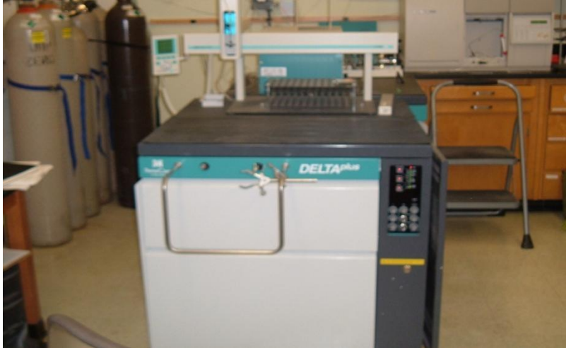
Figure 3. The Delta plus mass spectrometer used to analyze \delta^{15}\text{N} of water entrapped in filter.
