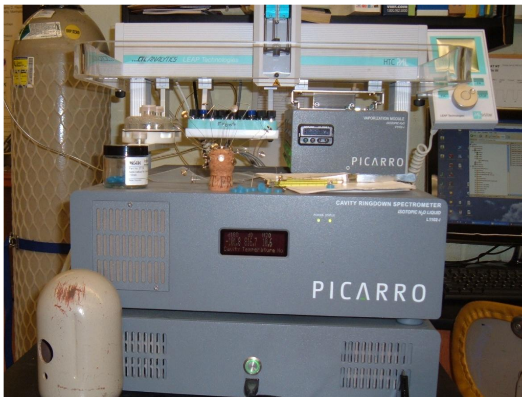
Figure 2. The Picarro G1301 used to analyze stable isotopes of \delta^2\text{H} and \delta^{18}\text{O} of water.
