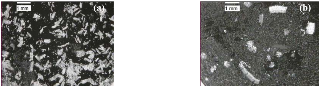
Figure 3.28 Chips of LAM at: (a)1480 °C and (b)1595 °C
