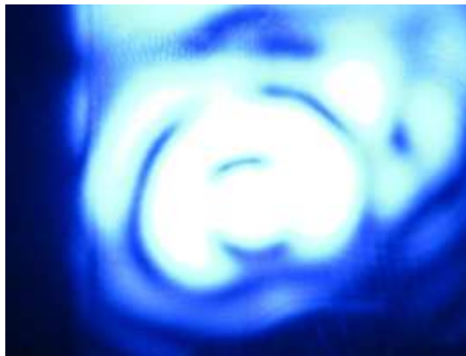
Figure 3-3 Beam profile of 400 nm pulses after the hollow core fiber
