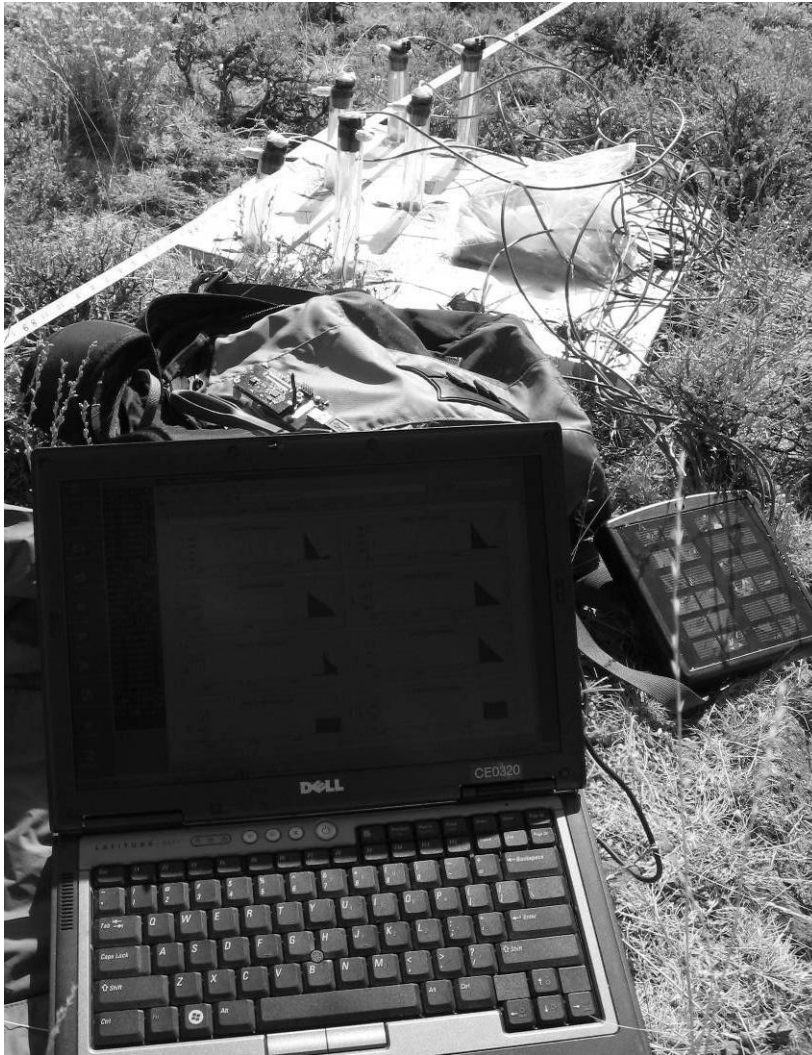
Figure 3.1. Automated mini-disk infiltrometers deployed in the field.
