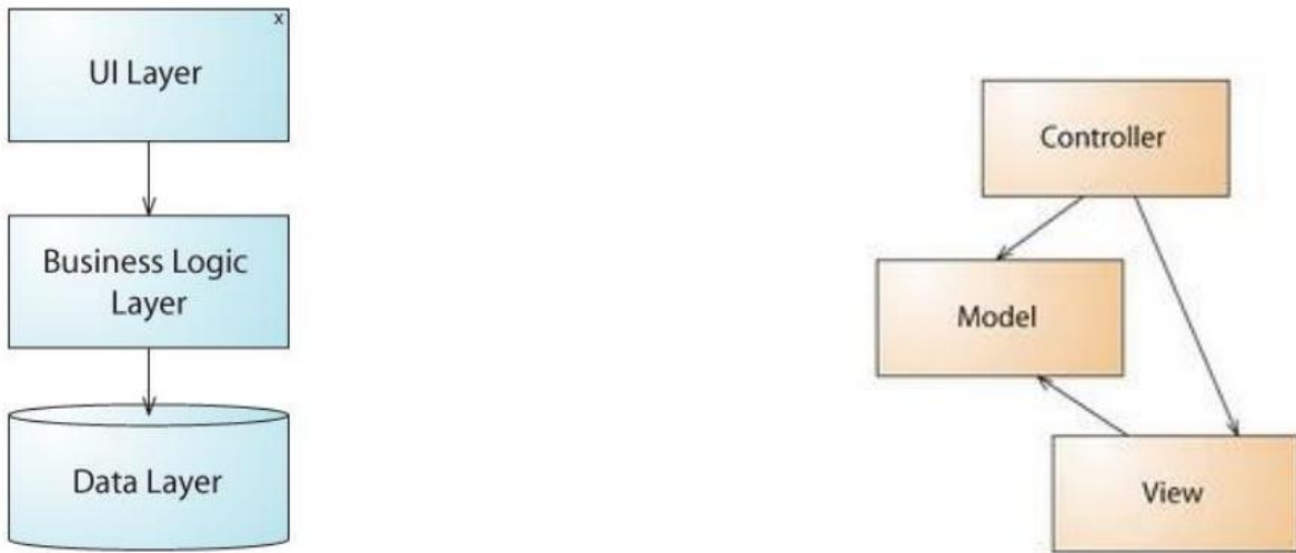
Figure 3.2 3-Tier VS MVC Architecture
