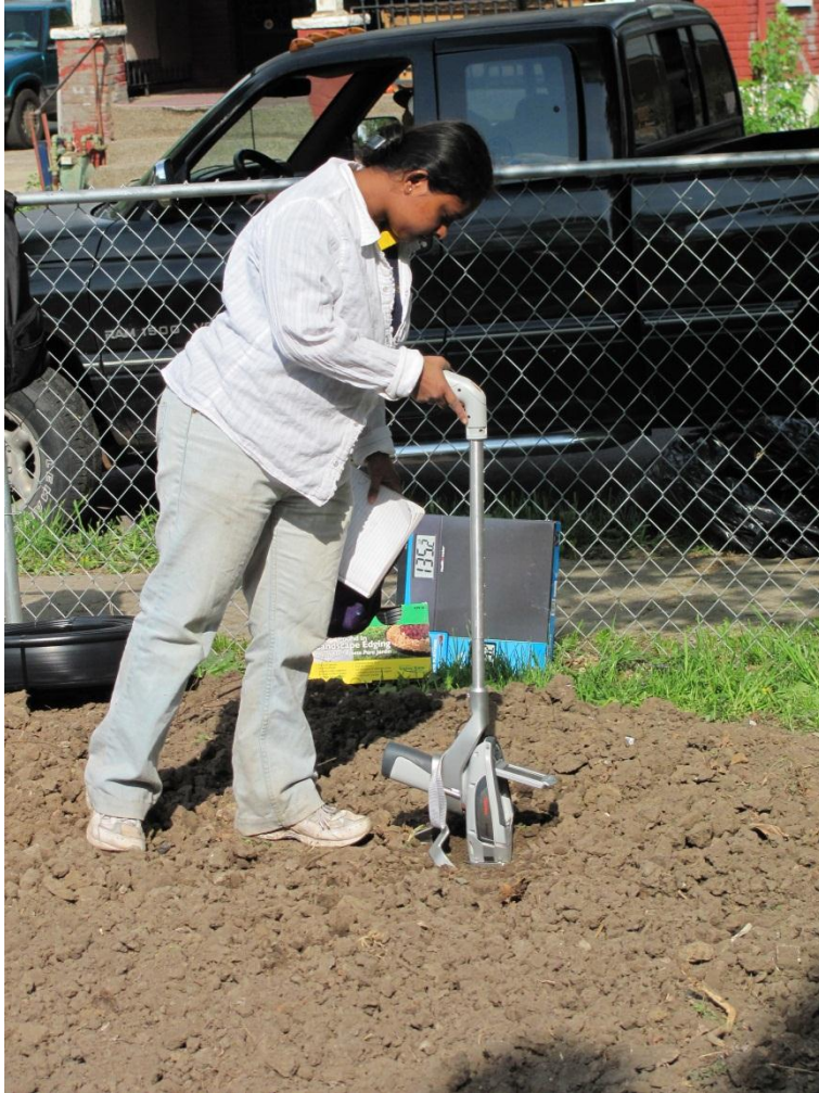
Figure 3.5 Conducting preliminary soil tests for total soil trace element concentrations on the Montgall Avenue vacant lot using the Field-Portable X-Ray Fluorescence Spectrophotometer.
