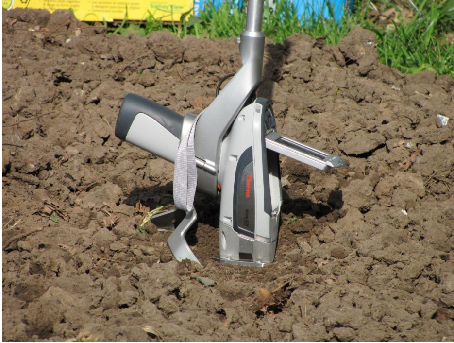
Figure 3.4 Field-portable X-Ray Fluorescence Spectrophotometer sampling for preliminary total soil trace element concentrations.
