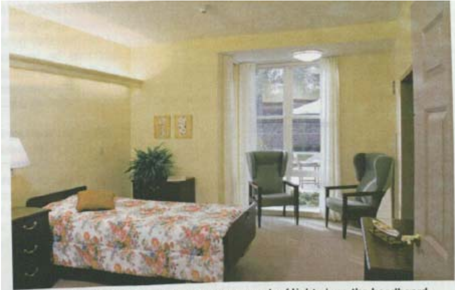
Figure 50. The light valance provides an even wash of light along the headboard wall. General ambient light is provided by the indirect light from the valance. The bedside table lamp provides additional task light for reading. The surface mounted ceiling light balances the luminance ratios between daylight and interior surfaces adjacent to the window. (© Jeffrey Totaro)
