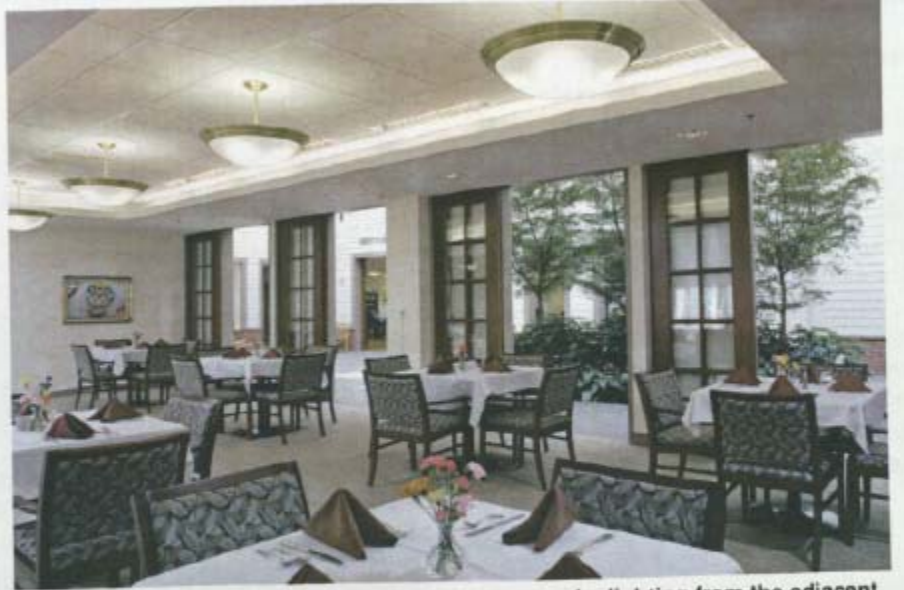
Figure 49. This dining area successfully integrates daylighting from the adjacent space with interior lighting provided by pendant indirect luminaires and cove lighting to provide diffused ambient light. Good contrast is provided by dark chairs against a medium value carpet and eating utensils against a white tablecloth. (© Jeffrey Totaro)
