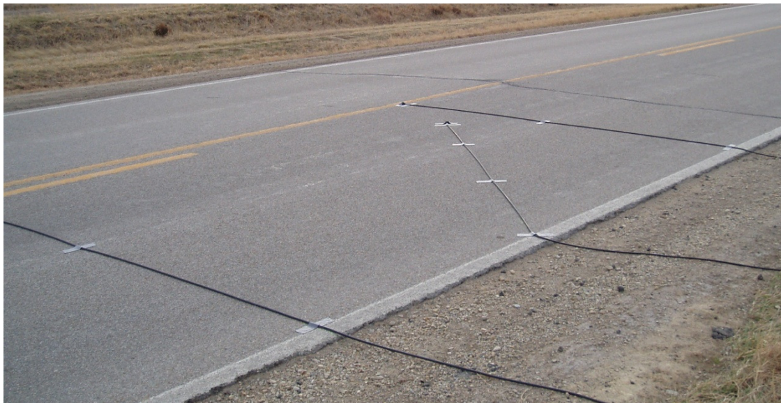
Figure 5.5 “Z” Configuration of Sensors for Data Collection
