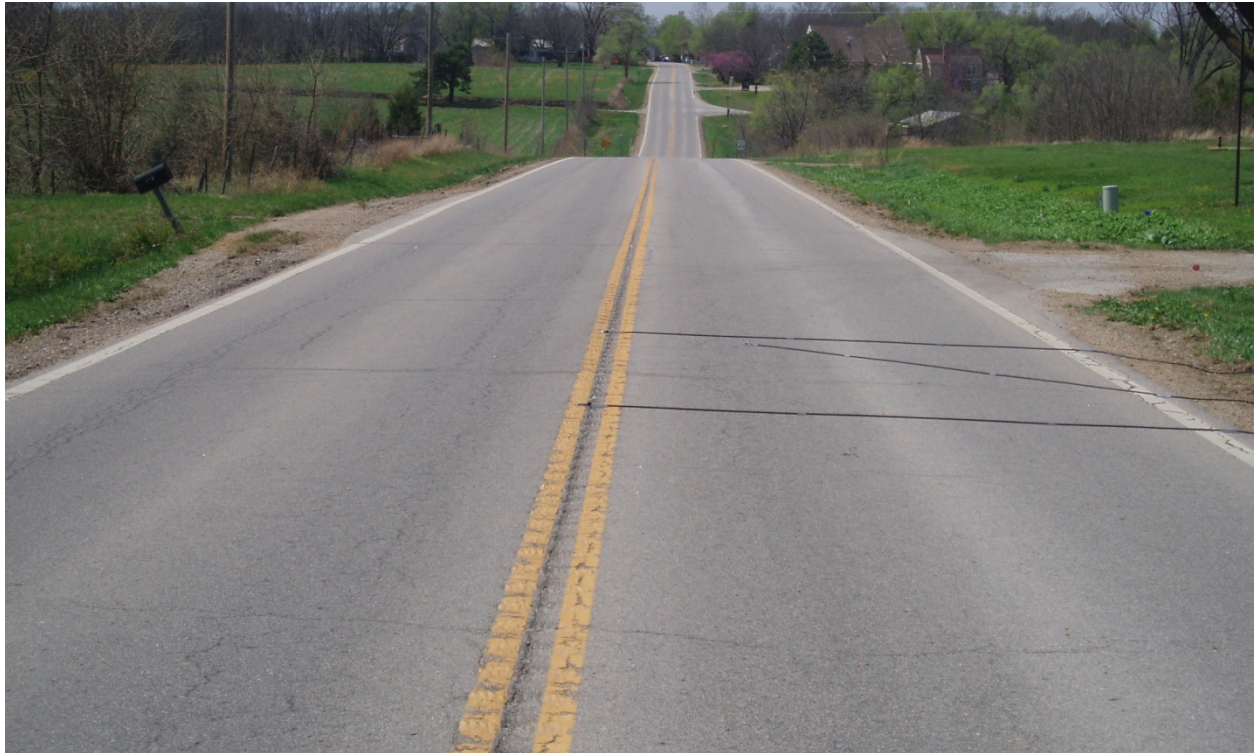
Figure 5.5 “Z” Configuration of Sensors for Data Collection
