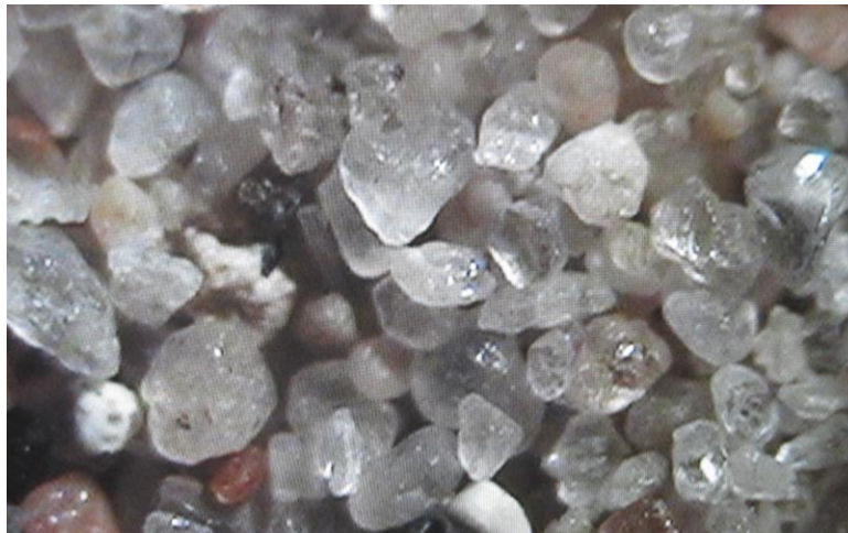
Figure 5-43: Magnified Image of \chi_l = 0\% , w = 0\% (dry sand)
