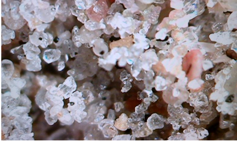
Figure 5-44: Magnified Image of \chi_l = 0\% , w = 4\% (moist sand)
