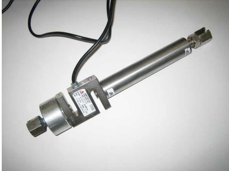
Figure 4-3: Photograph of “S” Type Load Cell
