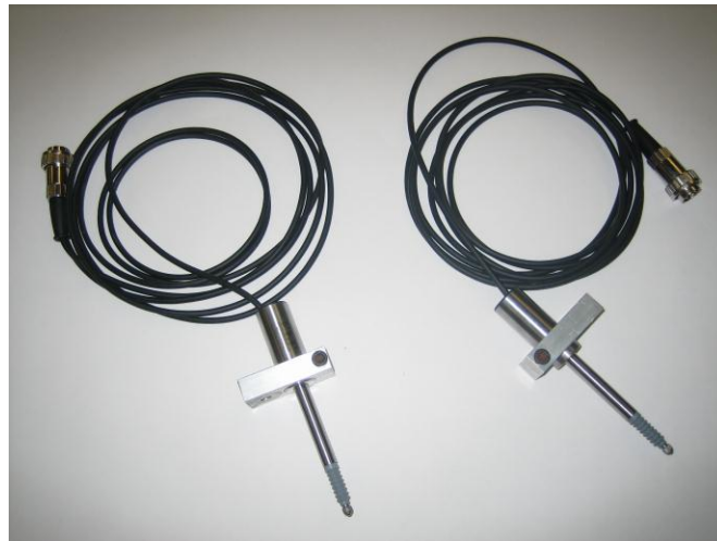
Figure 4-2: Photograph of Linear Variable Displacement Transducers
