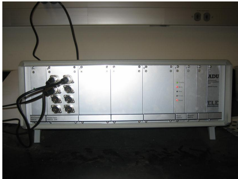
Figure 4-5: Photograph of Autonomous Data Acquisition Unit
