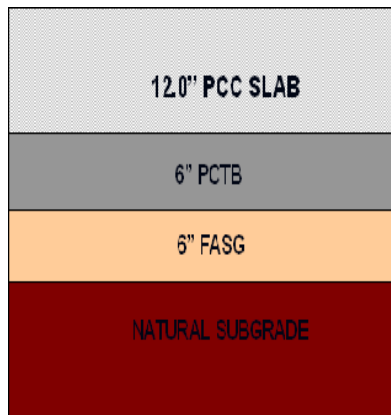
(c) SPS-2 Control Section
