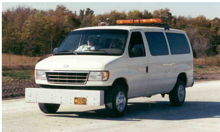
Figure 2.18 KDOT South Dakota-type profilometer
