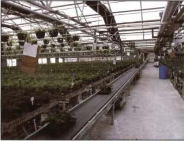
Figure 7-1. A permanent conveyor speeds flat movement at Tagawa Greenhouses in Brighton, Colorado. (Photo by Williams)
