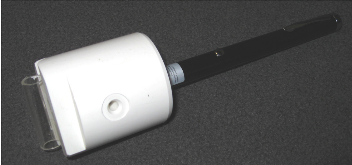
Figure 3-3: Modified green laser pointer to create a light sheet
