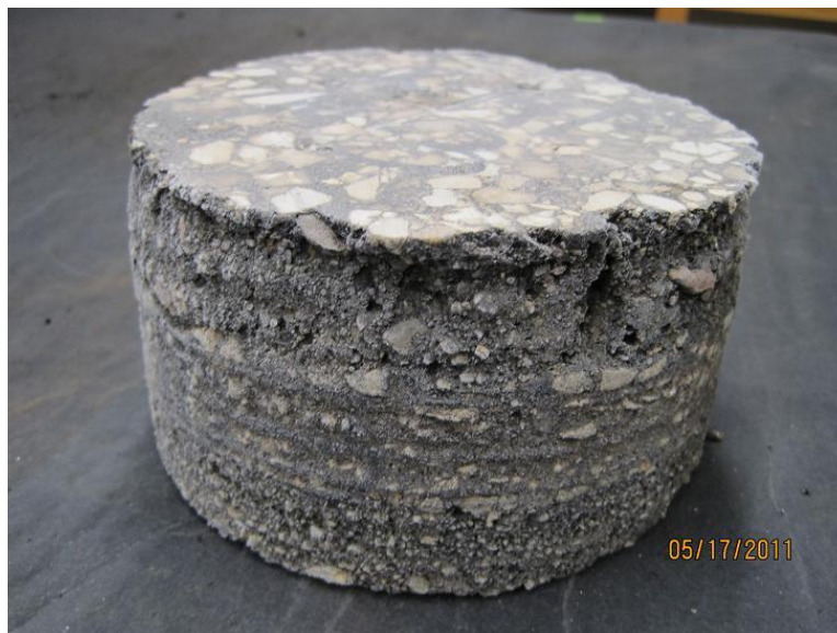
Figure 4.1 Typical IDT specimen for K-141 showing moderate stripping
