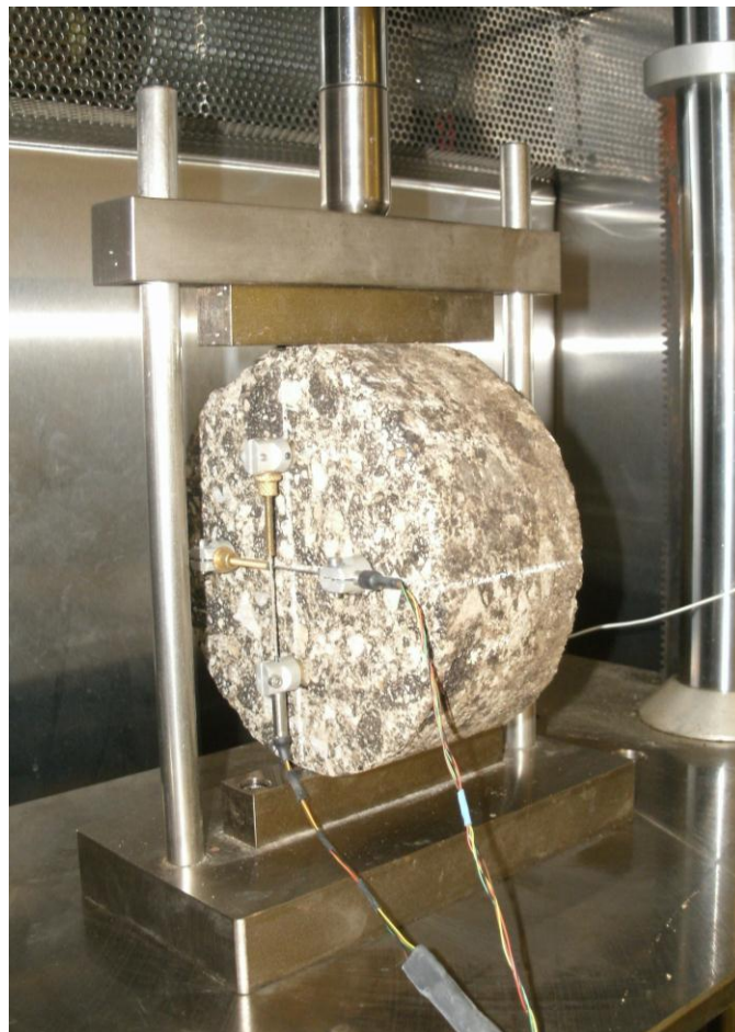
Figure 3.5 AASHTO TP-9 Setup
