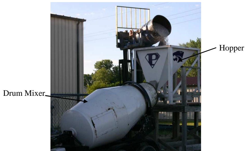
Figure 3.7 Adding Aggregates to Mixer
