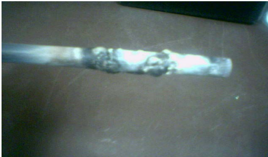
Figure 5-91 Photograph of the failed test heater for lithium metaborate deposition test at 1000 psia fluid pressure
