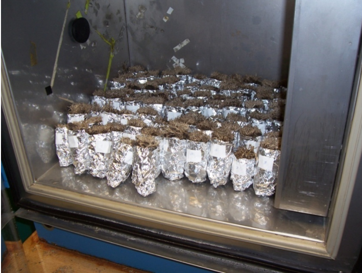
Figure 2.1- Samples in a thermocontrolled freezer preparing to undergo freeze tolerance testing.
