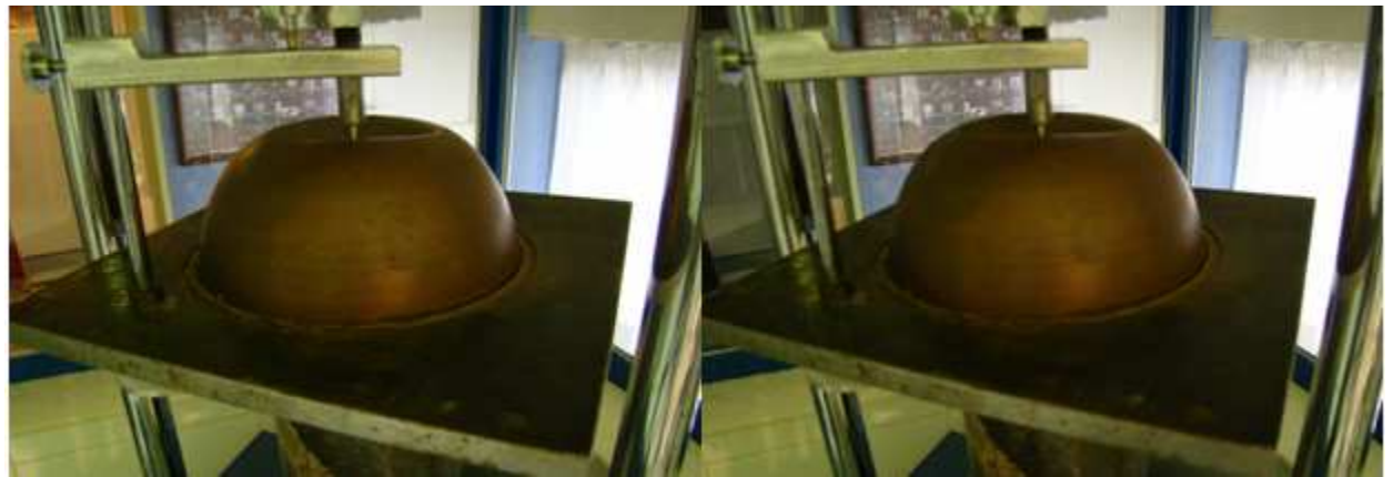
Figure 1. 25: Deformation of the moderately thick shell (Copper alloy R/t_0 \approx 75 )
