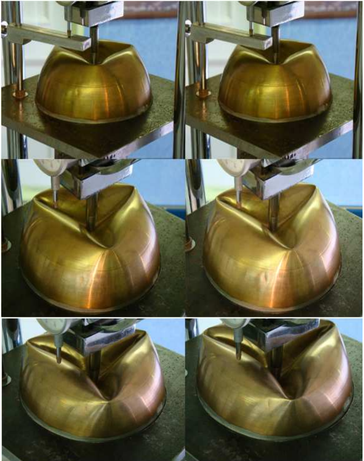
Figure 1. 31: Secondary bifurcation deformation of the thin shell (Bronze R/t_0 \approx 250 )
