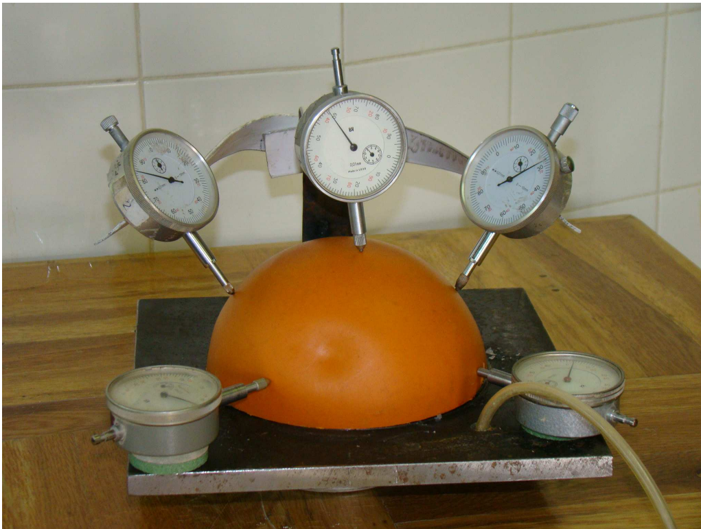
Figure 2. 33: Initial buckling of hemispherical shells under uniform suction pressure ( R= 75 mm).
