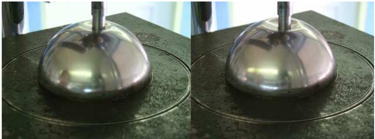
Figure 1. 26: Initial buckling and post buckling of the thin shell (Stainless Steel R/t_0 \approx 166 ).
