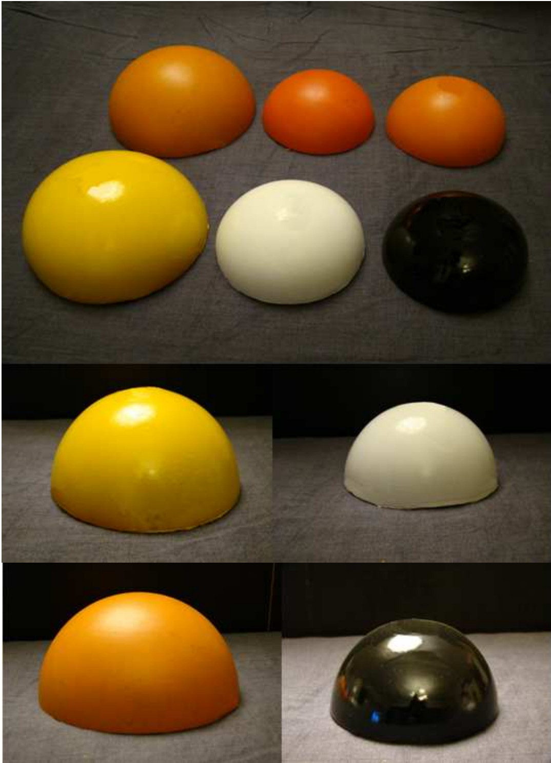
Figure 2. 26: Hemispherical shells samples made of polyethylene
