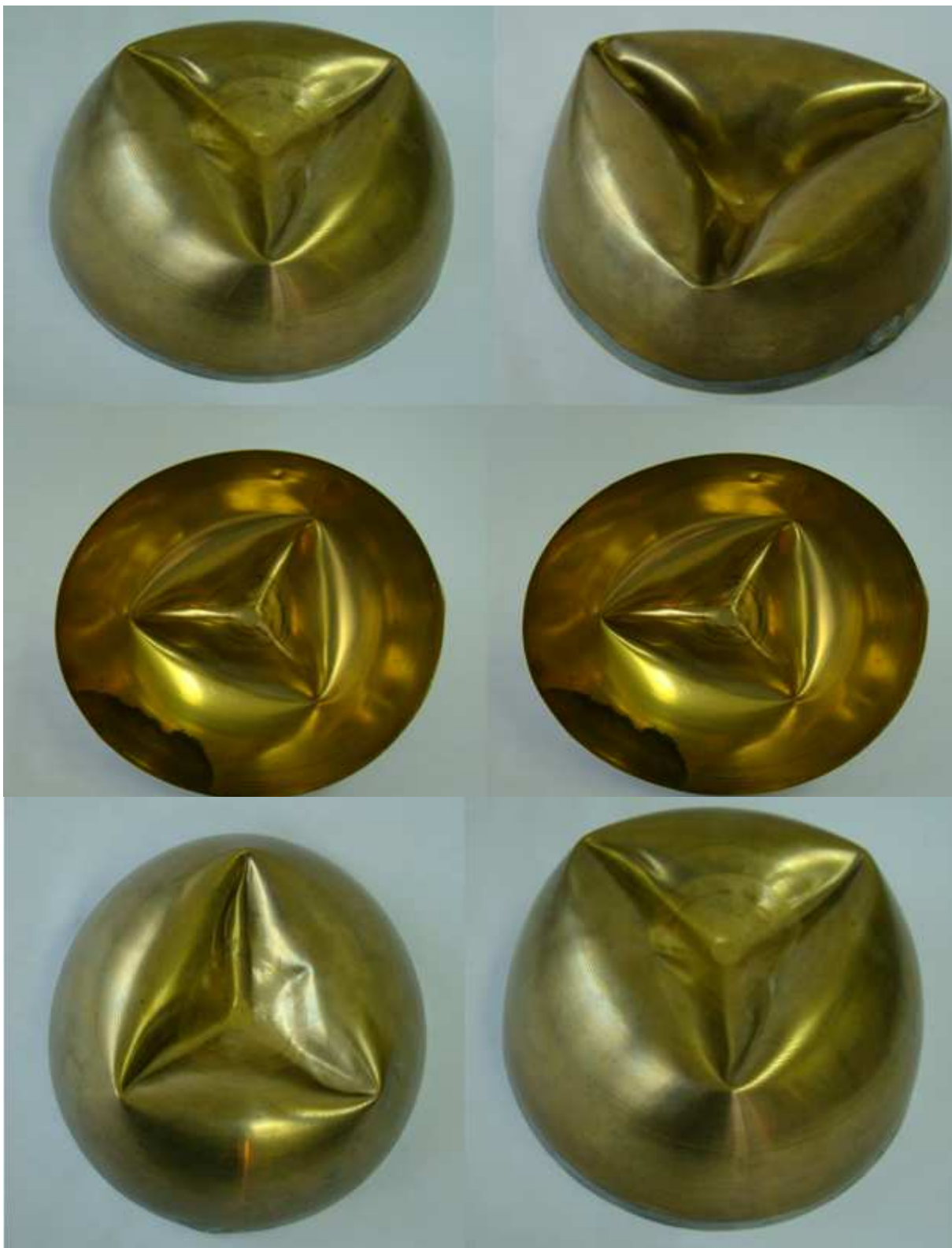
Figure 1. 32: Different stages of the triangular with secondary bifurcation (Bronze R/t_0 \approx 250 )
