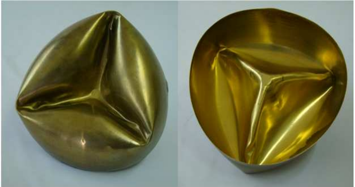
Figure 1. 33: Final deformation of the thin shell (Bronze R/t_0 \approx 250 )
