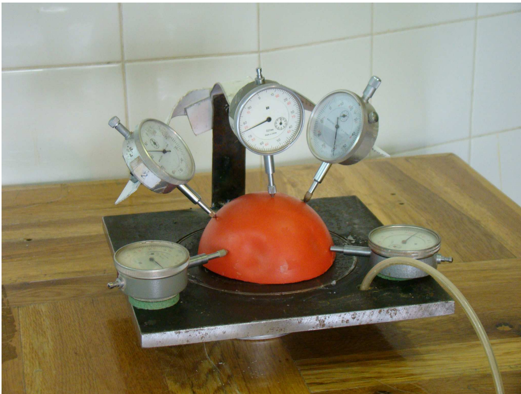
Figure 2. 31: Initial buckling of hemispherical shells under uniform suction pressure ( R= 50 mm).
