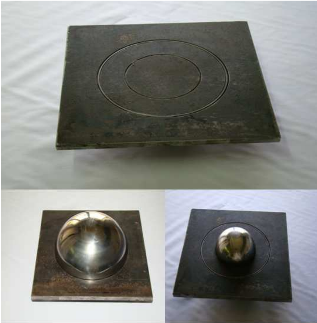
Figure 1. 20: Grooved base plate as a support for two sizes of hemispherical shells
