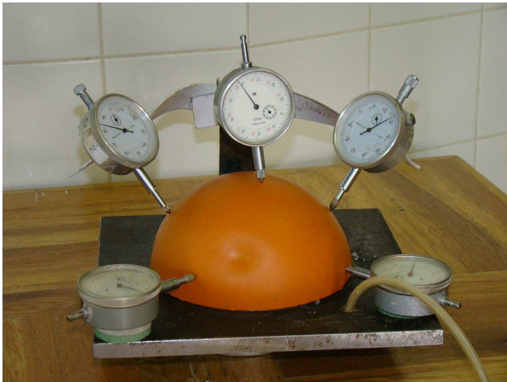
Figure 2. 34: Several tests made on different samples using suction pressure with three and five gages at different locations.
