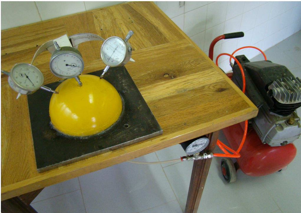
Figure 2. 27: A test made of R=75 mm shell using suction pressure and three displacement gages at various points.
