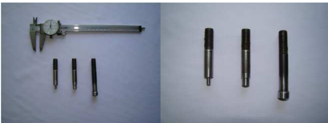
Figure 1. 19: Three different boss size used for loading ( b = 1.25, 2.5, 5.0 \text{ mm} )
