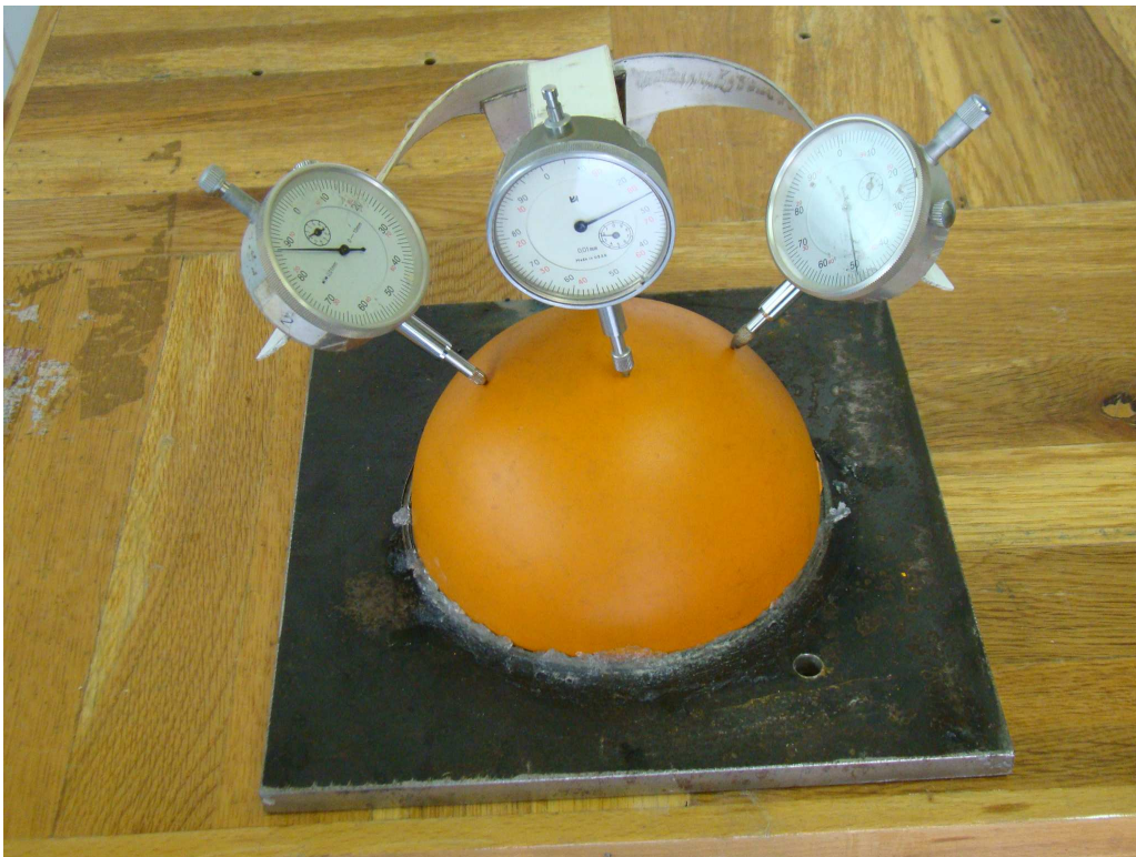
Figure 2. 28: Deformation measurement with three gauges at different locations in hemispherical shells under uniform suction pressure ( R= 75\text{mm} ).
