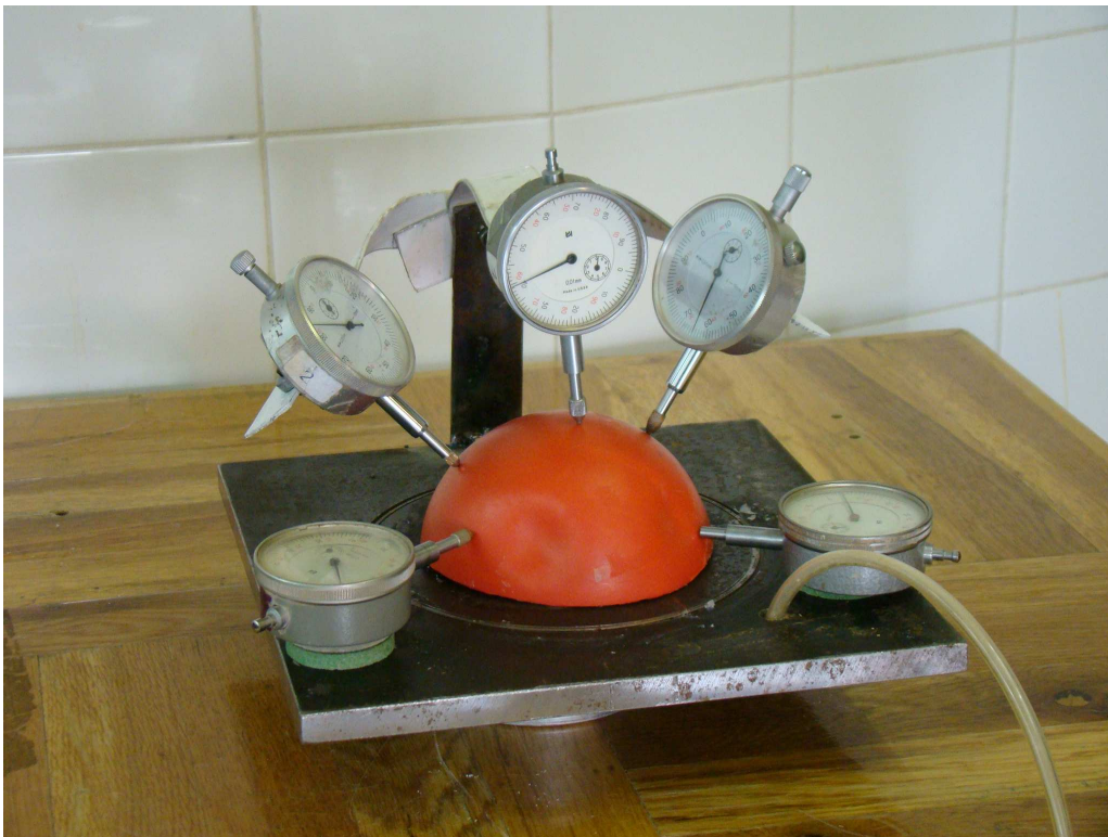
Figure 2. 32: Initial buckling of hemispherical shells under uniform suction pressure ( R= 50 mm).
