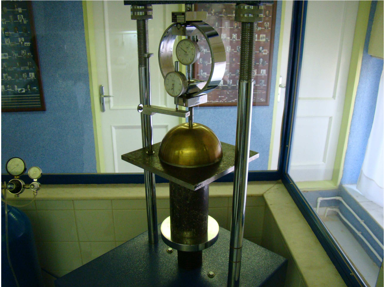
Figure 1. 21: Riehle Universal testing machine for displacement control measurements
