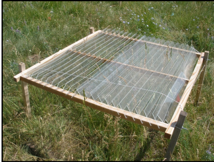
Figure 4-1 A louvered OSC as developed by Germino (personal communication). The optix plexi-glass slats reduce the loss of re-radiated daytime heat that occurs during the night, increasing nighttime temperature in the canopy.
