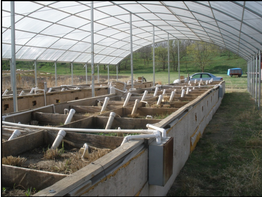
Figure 3-2 Rainfall Mesocosm Facility containing 64, 2.5m 3 cells under an 11 x 25 m rainout shelter.
