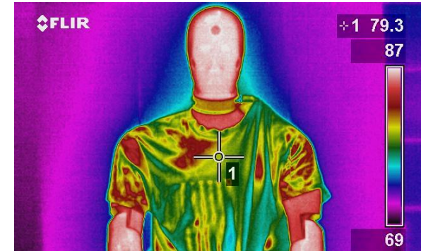
Bomb with Hot Pack Attached to Manikin at 150 Minutes
