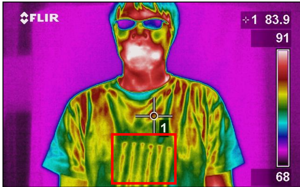
Figure 40—Bomb with Hot Pack Attached to Human at 1 Hour 40 Minutes
