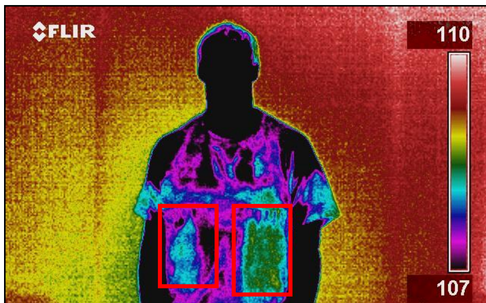
Figure 88—Metal Package Hidden in Vest Shielded by 2 Loose T-Shirts -Manual Temperature Range Setting
