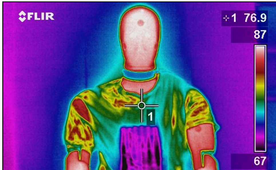
Figure 16—Bomb with Cold Pack Attached to Manikin at 0 Minutes
