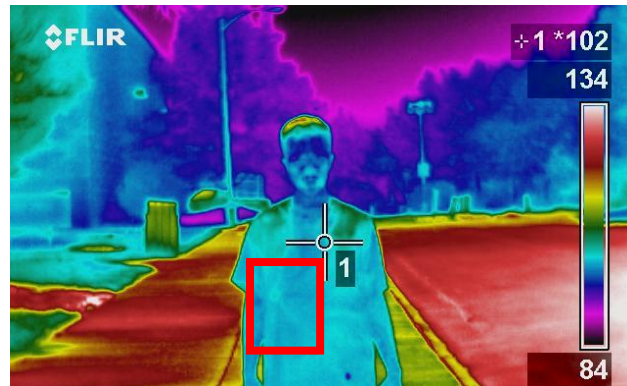
Walking Outside with Plastic Bomb at 1.0 Miles Automatic Temperature Scale Setting
