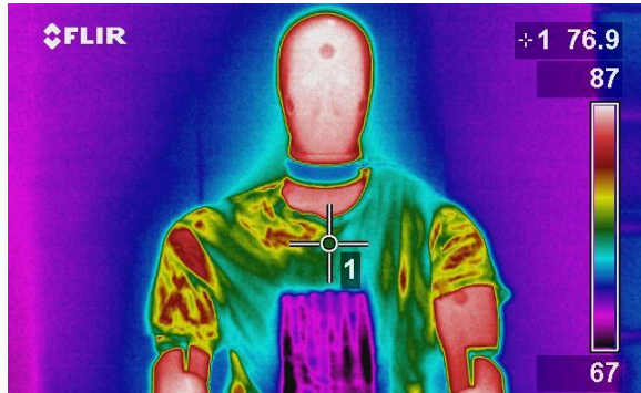
Bomb with Hot Pack Attached to Manikin at 0 Minutes
