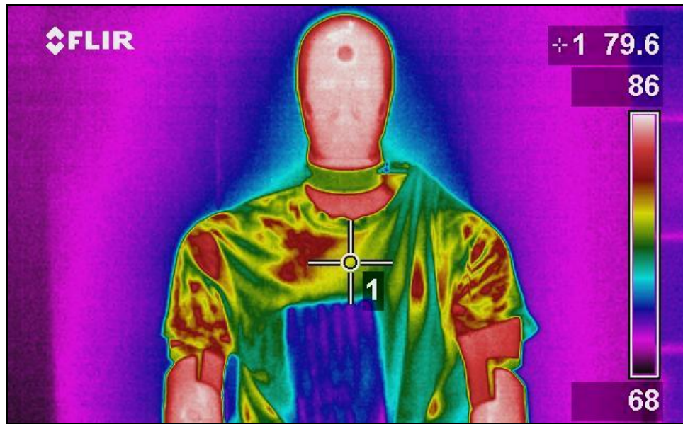
Figure 20—Bomb with Hot Pack Attached to Manikin at 0 Minutes
