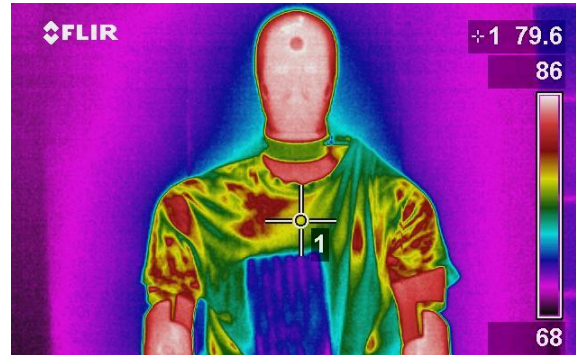
Bomb with Hot Pack Attached to Manikin at 90 Minutes
