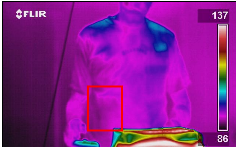
Figure 61—Walking on Treadmill with Plastic Bomb at 1.5 Miles
