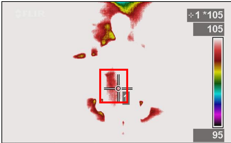
Figure 101—Walking Outside with Metal Bomb at 0.5 Miles - Manual Temperature Scale Setting
