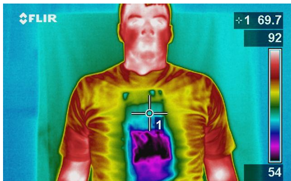
Bomb with Cold Pack Attached to Human at 0 Minutes
