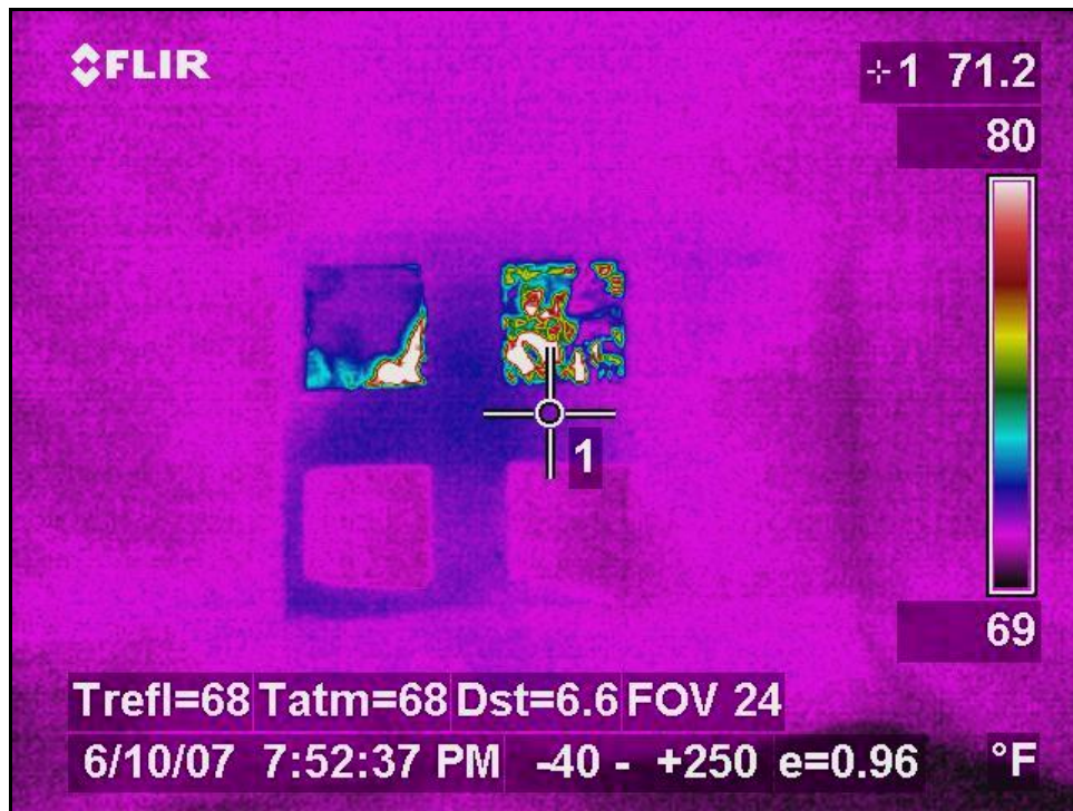
Figure 9—Material Coupons Top Row—Copper, Aluminum Foil, Blue Cotton Material Bottom Row—Paraffin Wax, Clay, Yellow Cotton Material
