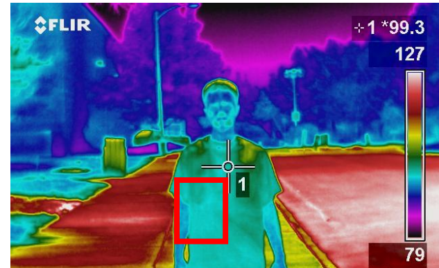
Walking Outside with Plastic Bomb at 0.5 Miles Automatic Temperature Scale Setting
