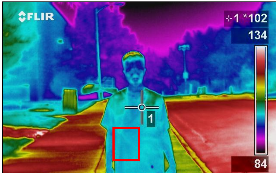
Figure 109—Walking Outside with Plastic Bomb at 1 Mile - Automatic Temperature Scale Setting
