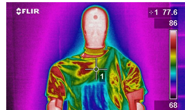
Bomb with Cold Pack Attached to Manikin at 180 Minutes
