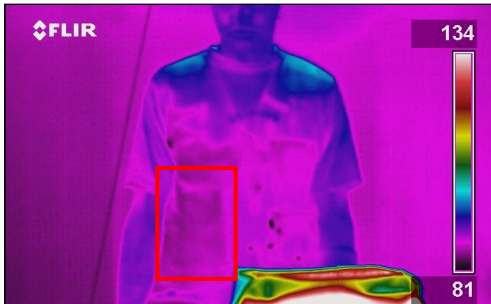
Figure 60—Walking on Treadmill with Plastic Bomb at 0 Miles
