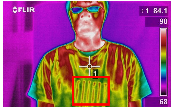
Bomb with Hot Pack Attached to Human at 27 Minutes
