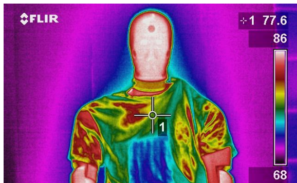
Bomb with Cold Pack Attached to Manikin at 0 Minutes
