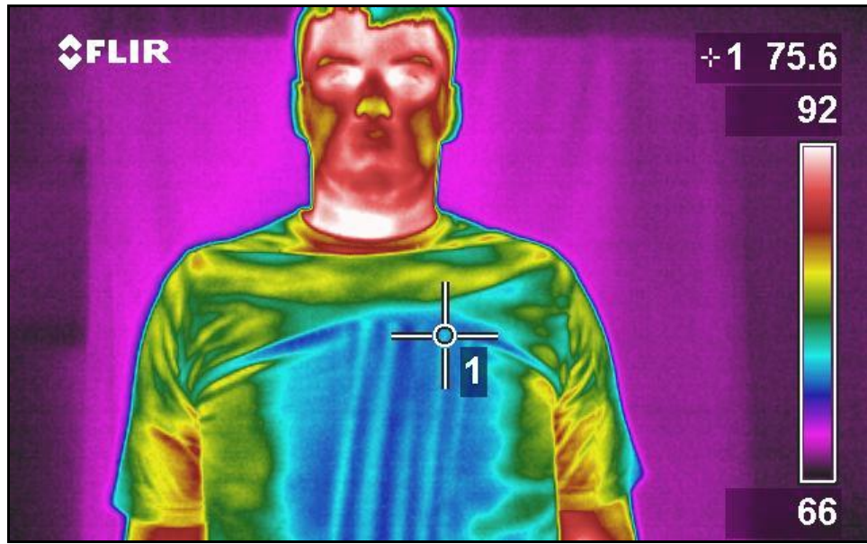
Figure 42—Bomb with Cold Pack Attached to Human at 1 Hour 30 Minutes
