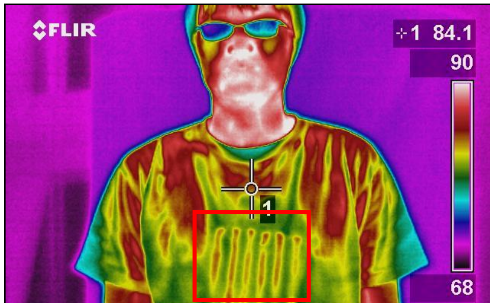
Figure 39—Bomb with Hot Pack Attached to Human at 27 Minutes
