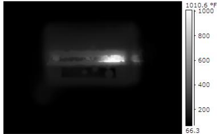
Figure 6.4 Image from Test 5 where CHF occurs only at the right side of the NiChrome surface.
