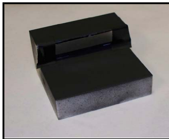
Figure A.2 Metallic strip placed on Teflon to establish a reflected temperature.
