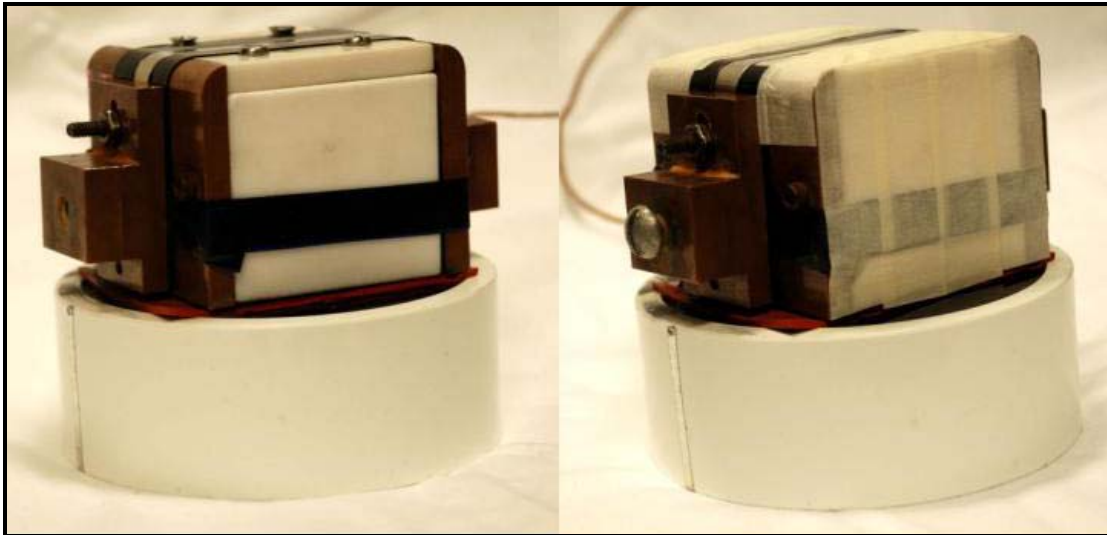
Figure 4.7: Photos of Heated Surface Assembly before (left) and after (right) masking tape is applied.
