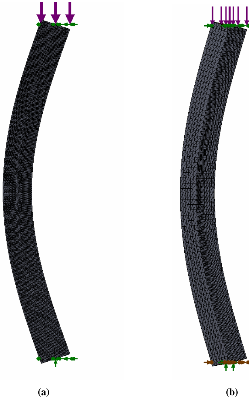
Figure 3.17 Initiation of Euler buckling in a (a) rhombic tube with l = 2 \text{ in} , t = 0.08 \text{ in} and \theta = 60^\circ at h = 23.5 \text{ in} and (b) parallelogram tube with l = 2 \text{ in} , l_r = 1 \text{ in} , t = 0.08 \text{ in} and \theta = 45^\circ at h = 9.5 \text{ in}
