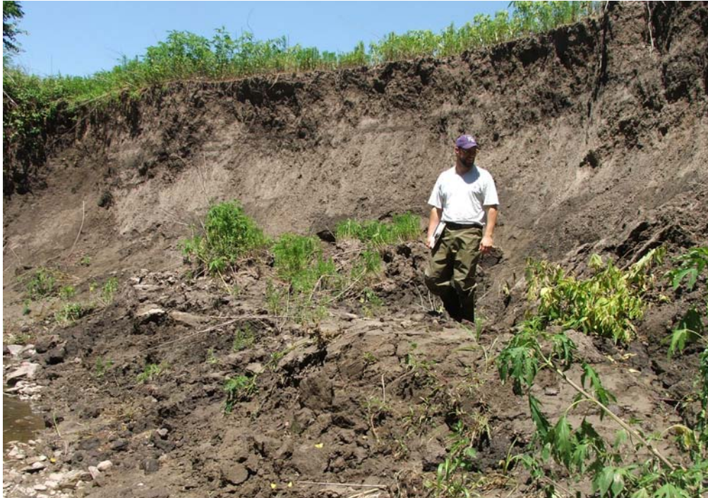
Figure 2.6 Irish Creek 2 study bank after June 2010 rains. Four-foot erosion pins were lost and the bank profile toe pin was buried (Keane, 2010).
