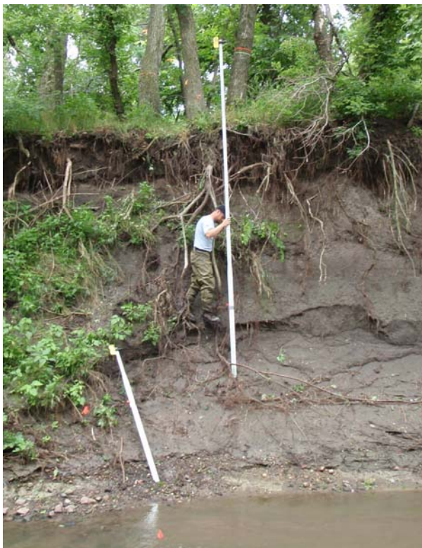
Figure 5.7 Main Stem study reach 3 illustrating vertical banks held together with woody vegetation root structure (Keane, 2010).
