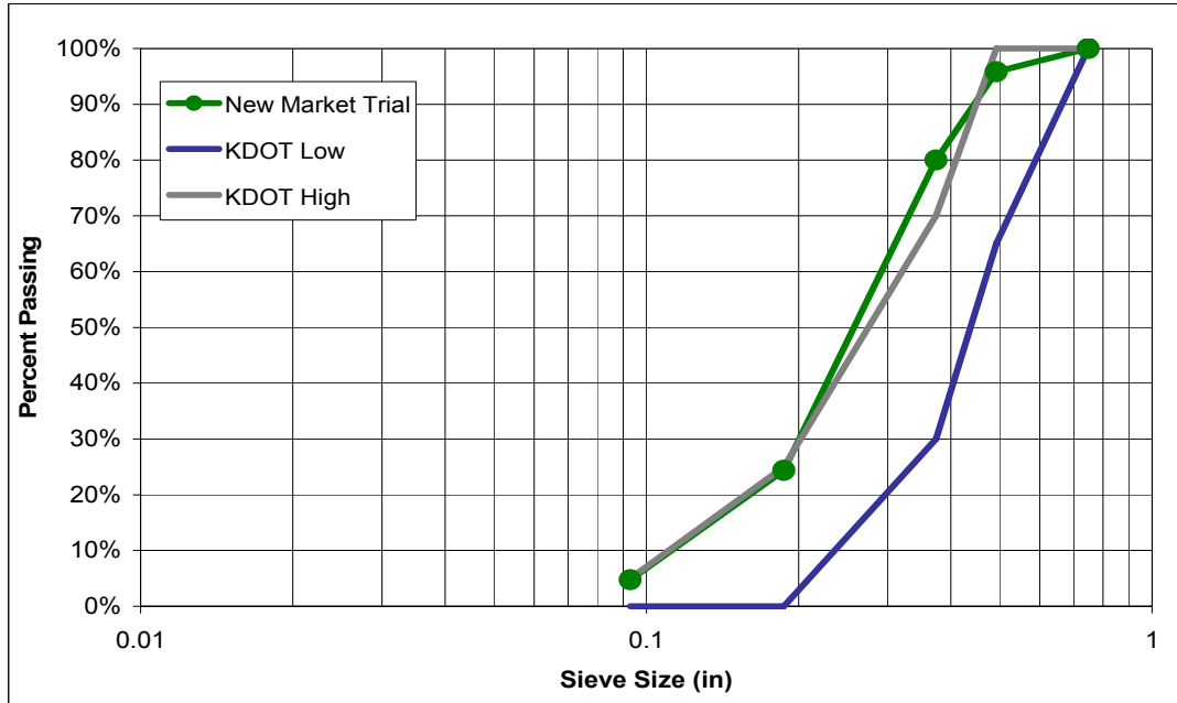
Figure 3.12. Gradation of New Market aggregate with KDOT CA-4 range.
