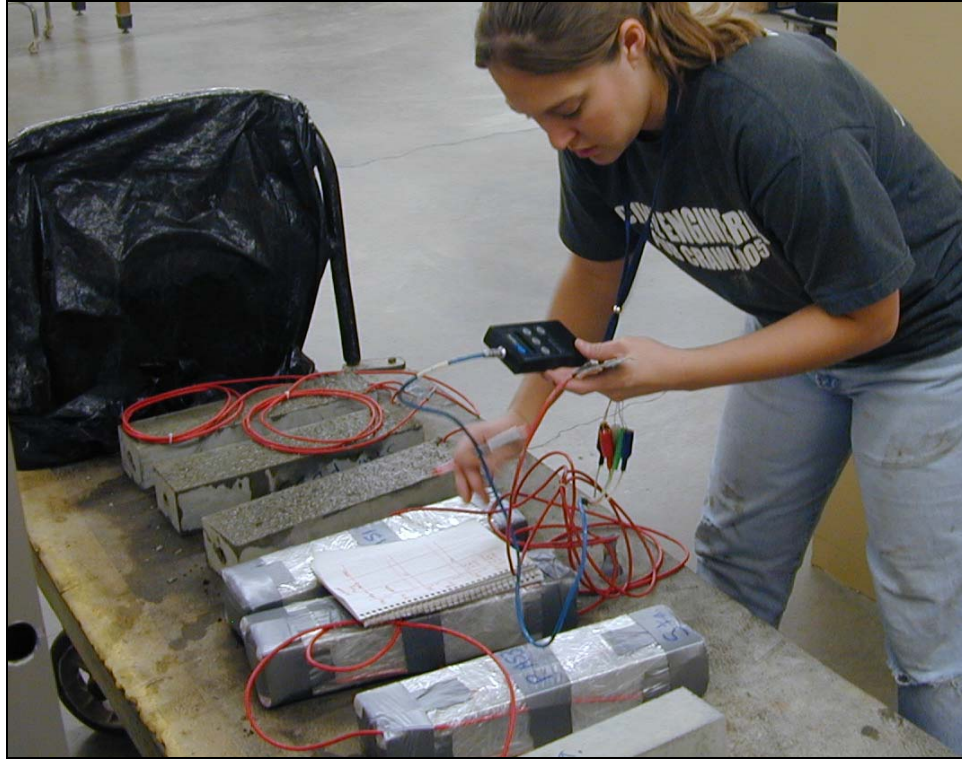
Figure 5.13. VWSGs being read in shrinkage beams.
