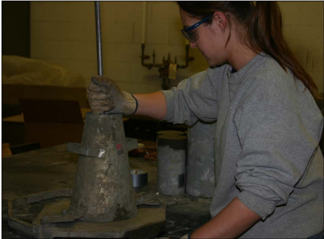
Figure 4.2. Conducting the slump test.
