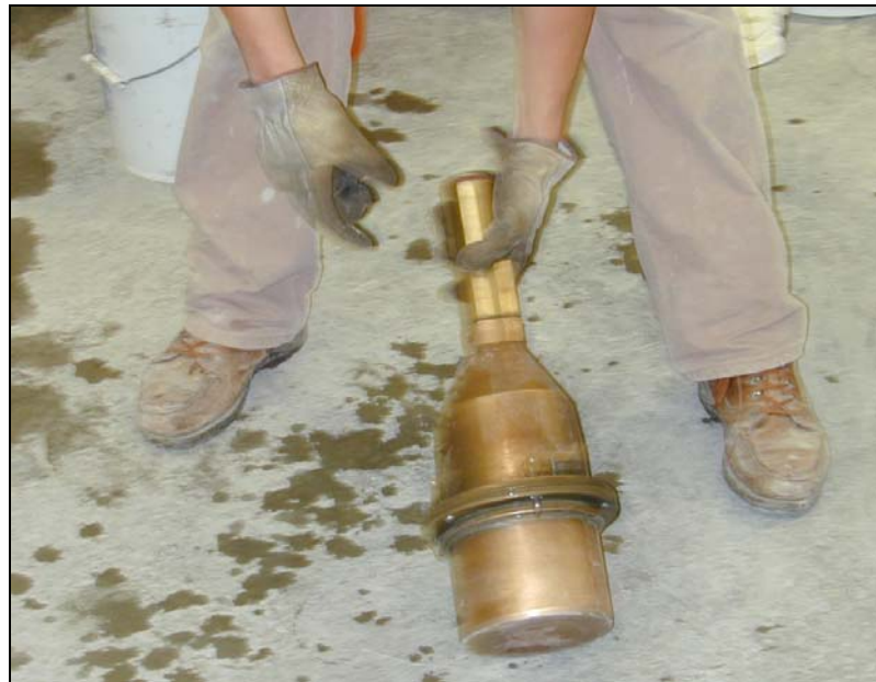
Figure 4.6. Agitating rollometer by rolling.
