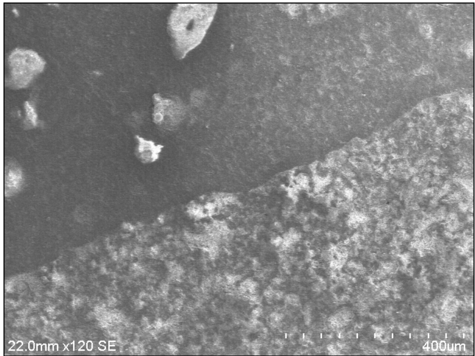
Figure 6.13. Stalite aggregate concrete with 400µm scale.
