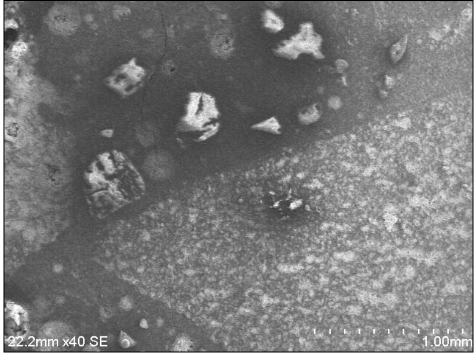
Figure 6.12. Contact zone of Stalite aggregate concrete with 1mm scale.
