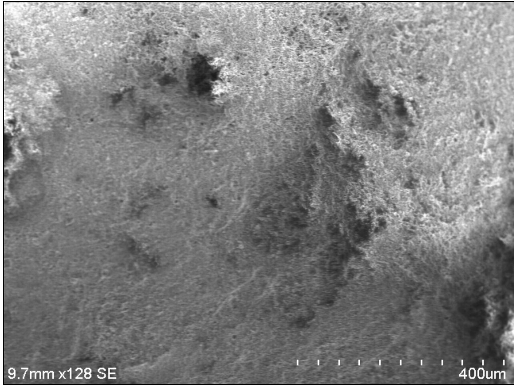
Figure 3.3. Marquette aggregate with 400µm scale using the scanning-electron microscope.
