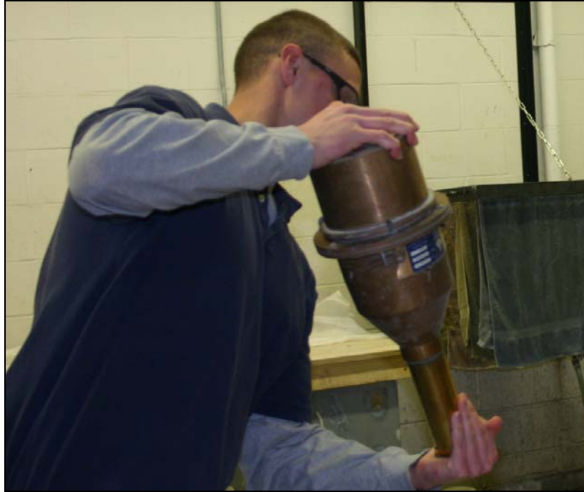
Figure 4.5. Agitating rollometer by inverting and shaking.
