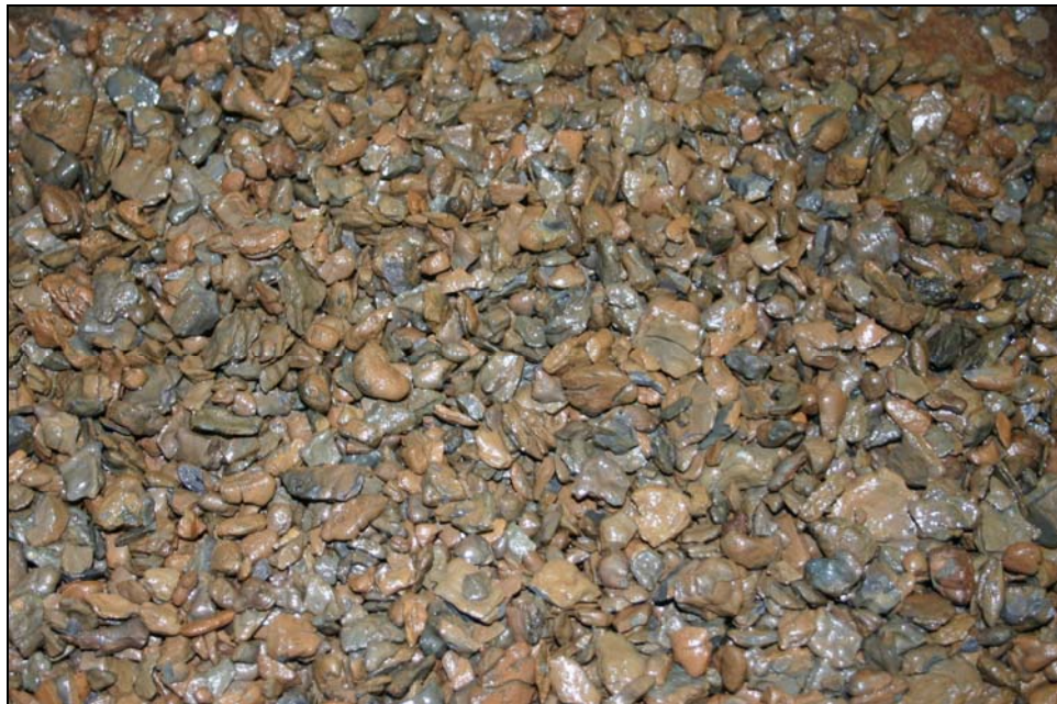
Figure 4.10. New Market aggregate in the wet condition.
