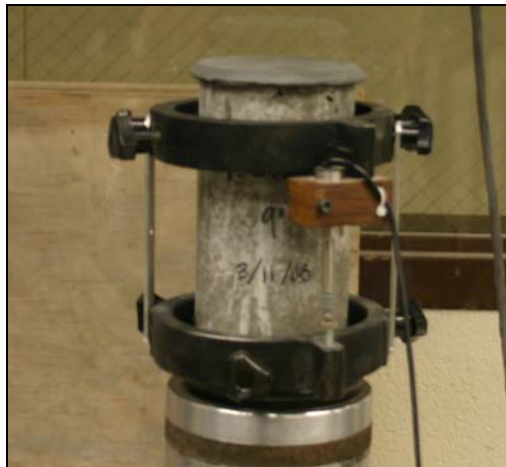
Figure 5.5 Compressometer setup for modulus of elasticity test.
