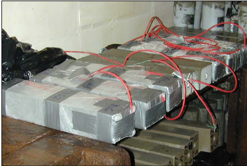
Figure 5.12. Wrapped and sealed autogenous shrinkage beams in moist room.
