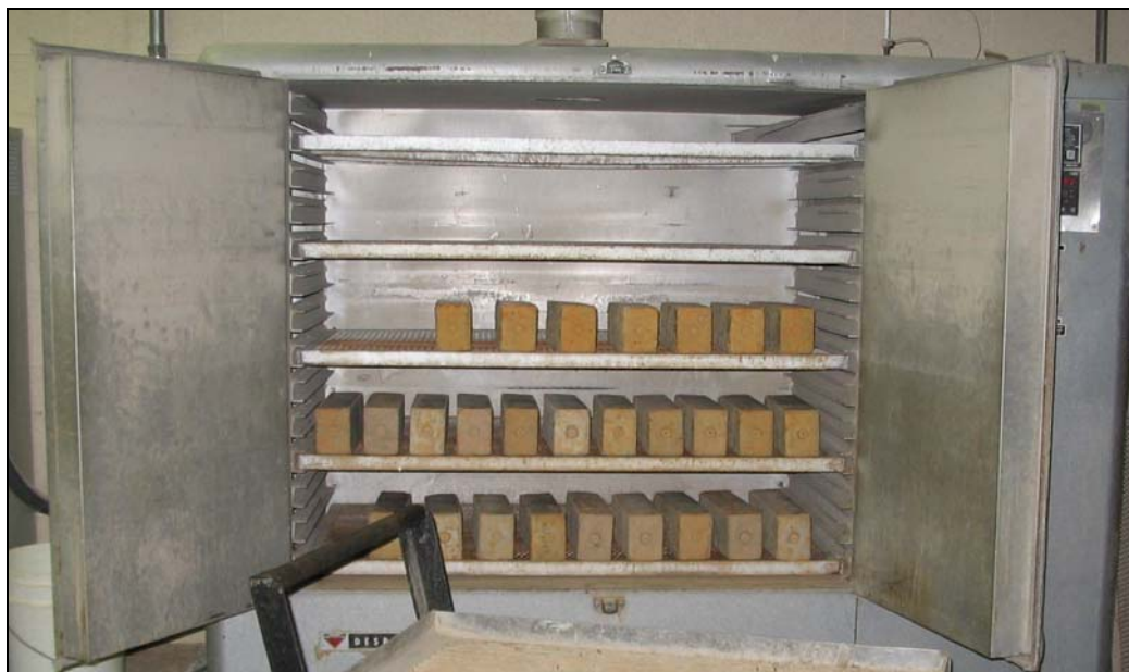
Figure 5.8. Alkali-silica reactivity test beams in oven.
