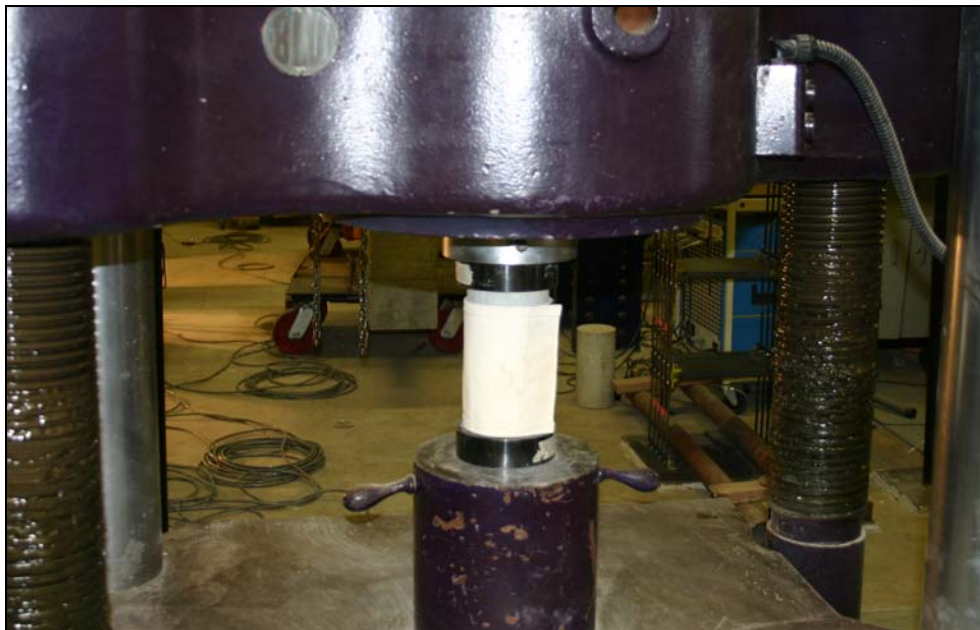
Figure 4.8. Testing a compressive cylinder with neoprene caps.
