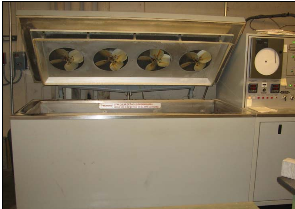
Figure 5.6. Freeze-thaw resistance testing apparatus.
