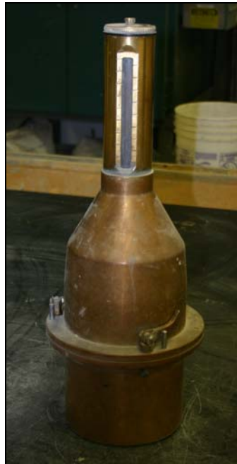
Figure 4.4. Rollometer used to determine volumetric air content.
