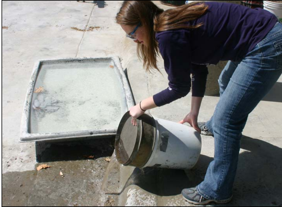
Figure 5.1. Water being strained for small concrete batch.
