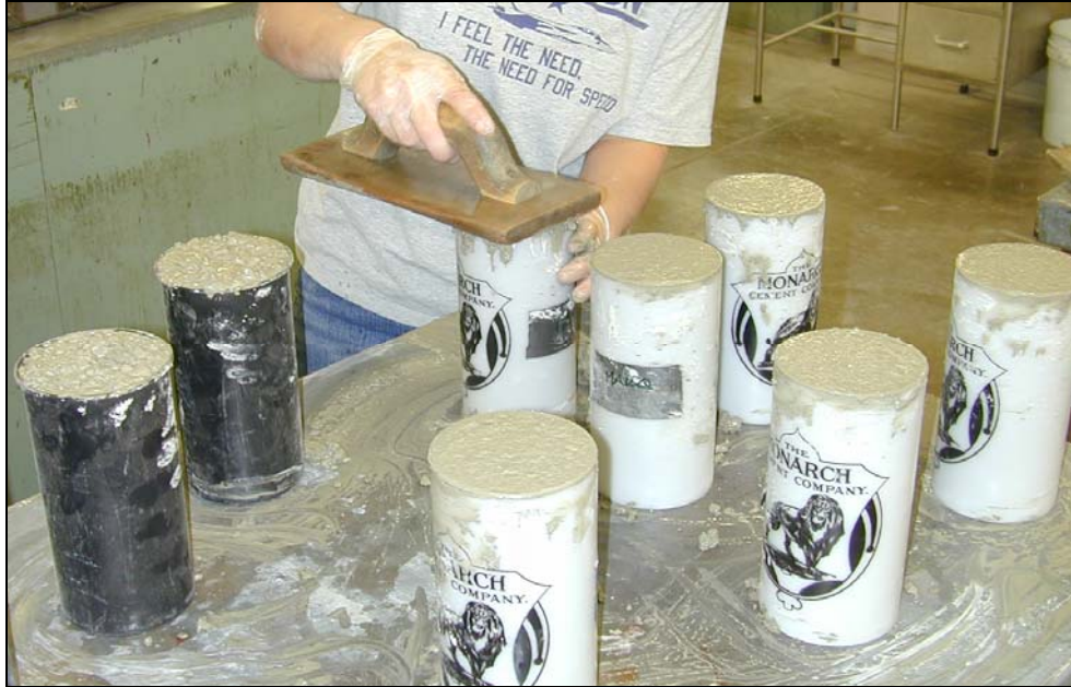
Figure 4.7. Making compressive cylinders.
