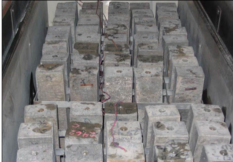
Figure 5.7. Freeze-thaw beams in testing tank.
