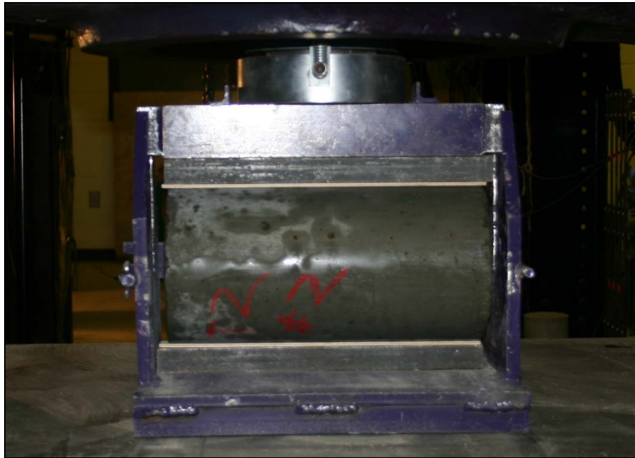
Figure 5.4. Splitting tensile strength test setup.
