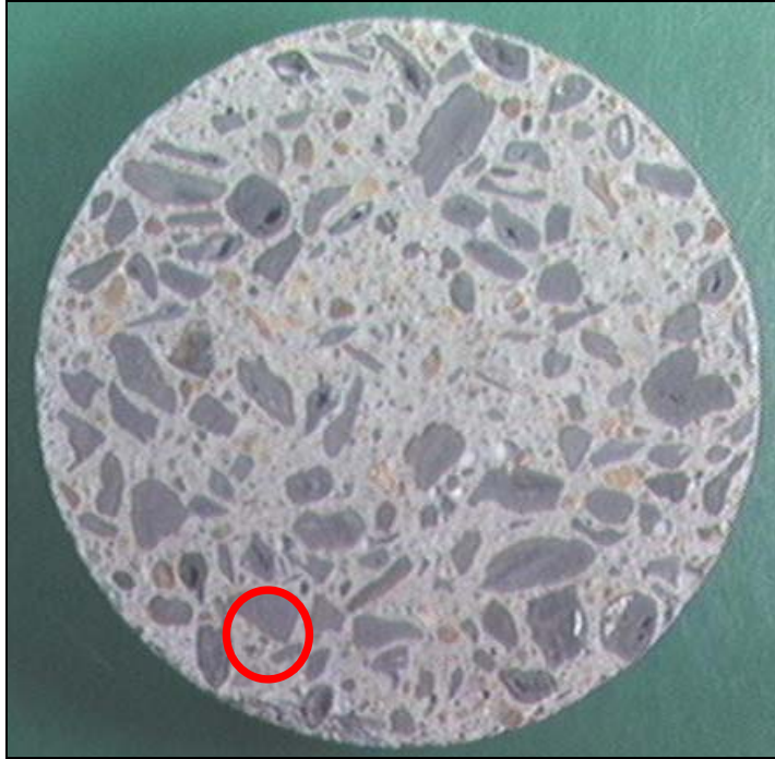
Figure 6.6. Polished cylinder cross-section of New Market aggregate concrete.
