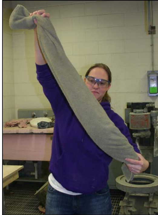
Figure 4.11. Drying wet aggregate to the saturated surface dry (SSD) condition.
