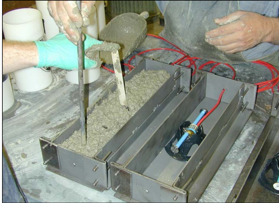
Figure 5.10. Shrinkage beams during casting with VWSGs.
