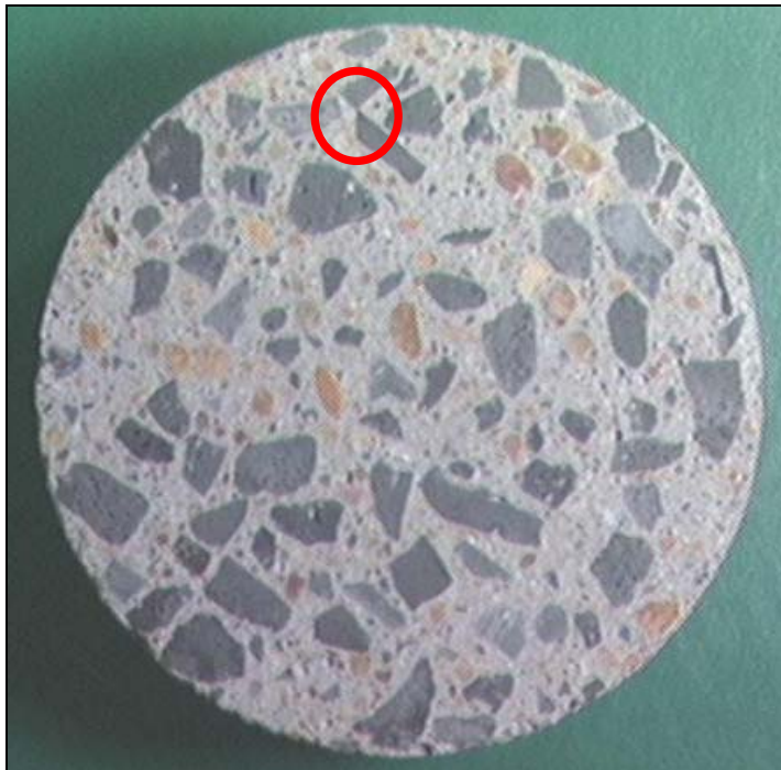
Figure 6.7. Polished cylinder cross-section of Stalite aggregate concrete.
