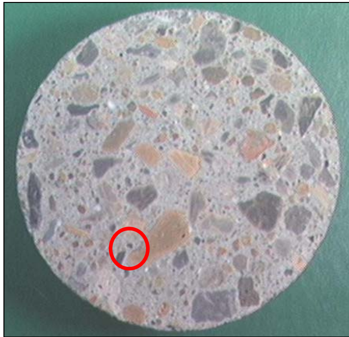
Figure 6.5. Polished cylinder cross-section of Marquette aggregate concrete.
