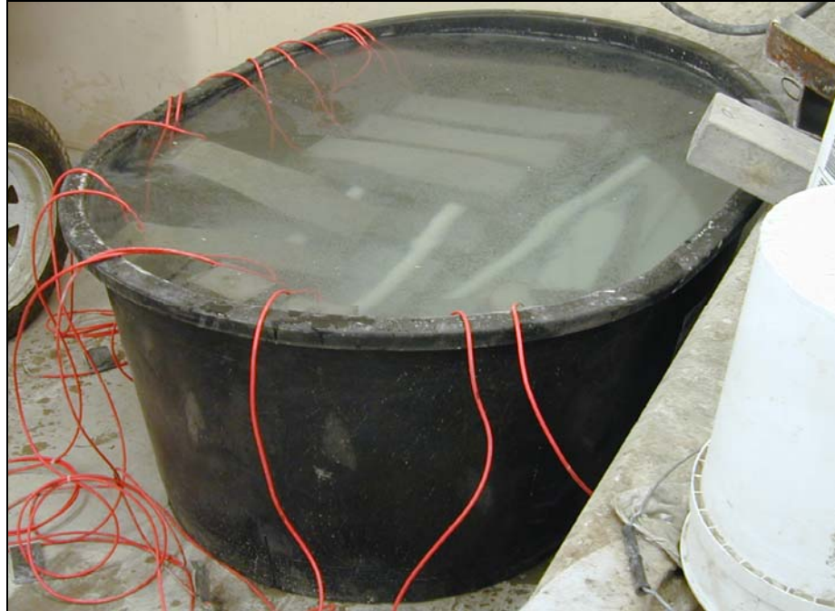
Figure 5.11. Lime water storage tank for drying shrinkage beams.
