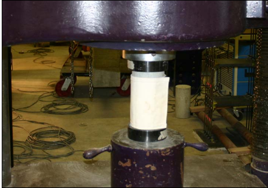
Figure 5.3. Compressive strength test setup.
