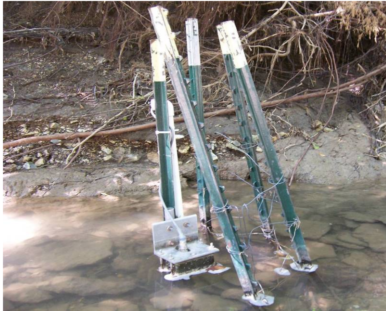
Figure 3.4 Sensor was mounted using heavy duty metal stakes (green T-post) at Little Kitten Creek, Manhattan, Kansas.
