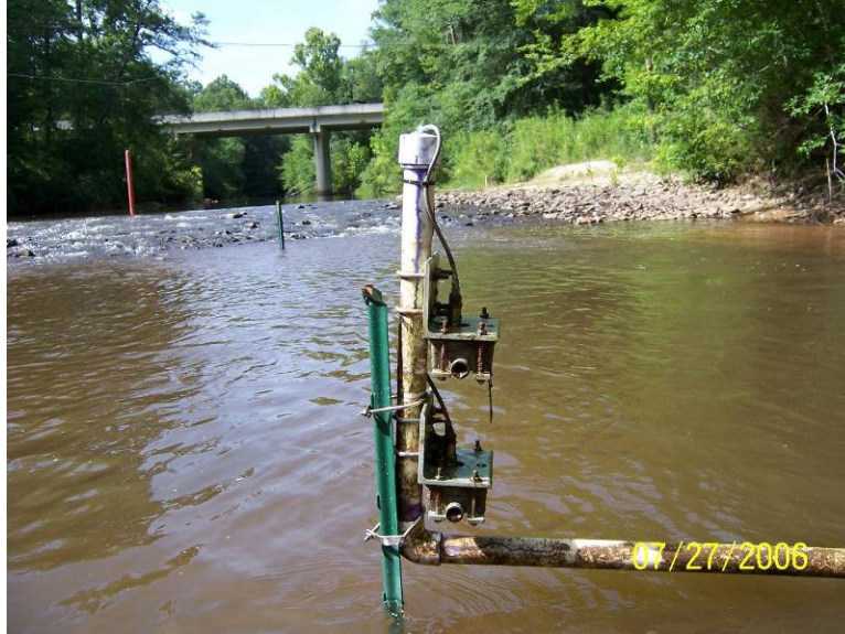
Figure 3.5 Sensors were mounted using PVC pipe and metal stakes (green T-post) at Fort Benning, Georgia.
