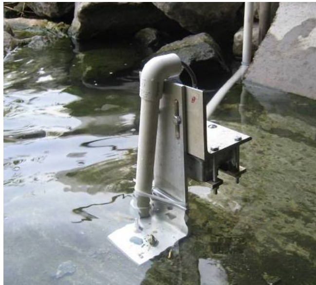
Figure 3.1 Sensor mounted using an L-shaped aluminum plate at Mission, Kansas.
