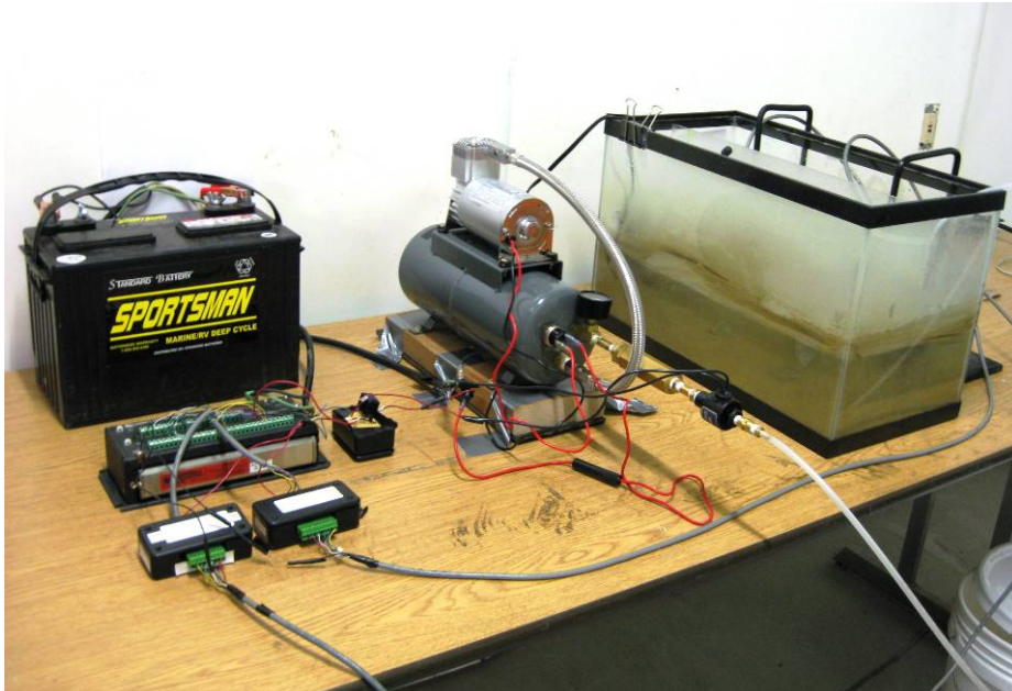
Figure 4.4 Laboratory setup of air-blast cleaning experiment.
