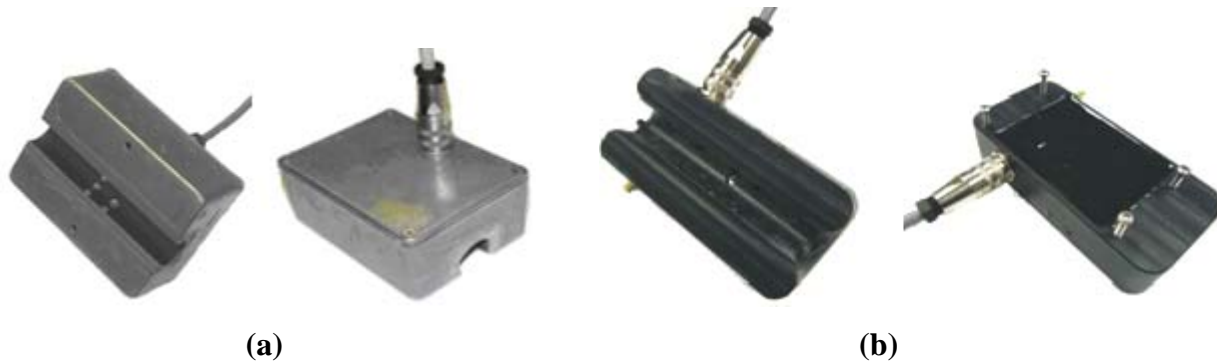
Figure 4.1 Two types of sensors used for cleaning experiments: (a) SSC sensor design with an aluminum case (2005); (b) SSC sensor design with a polyethylene case (2008)
