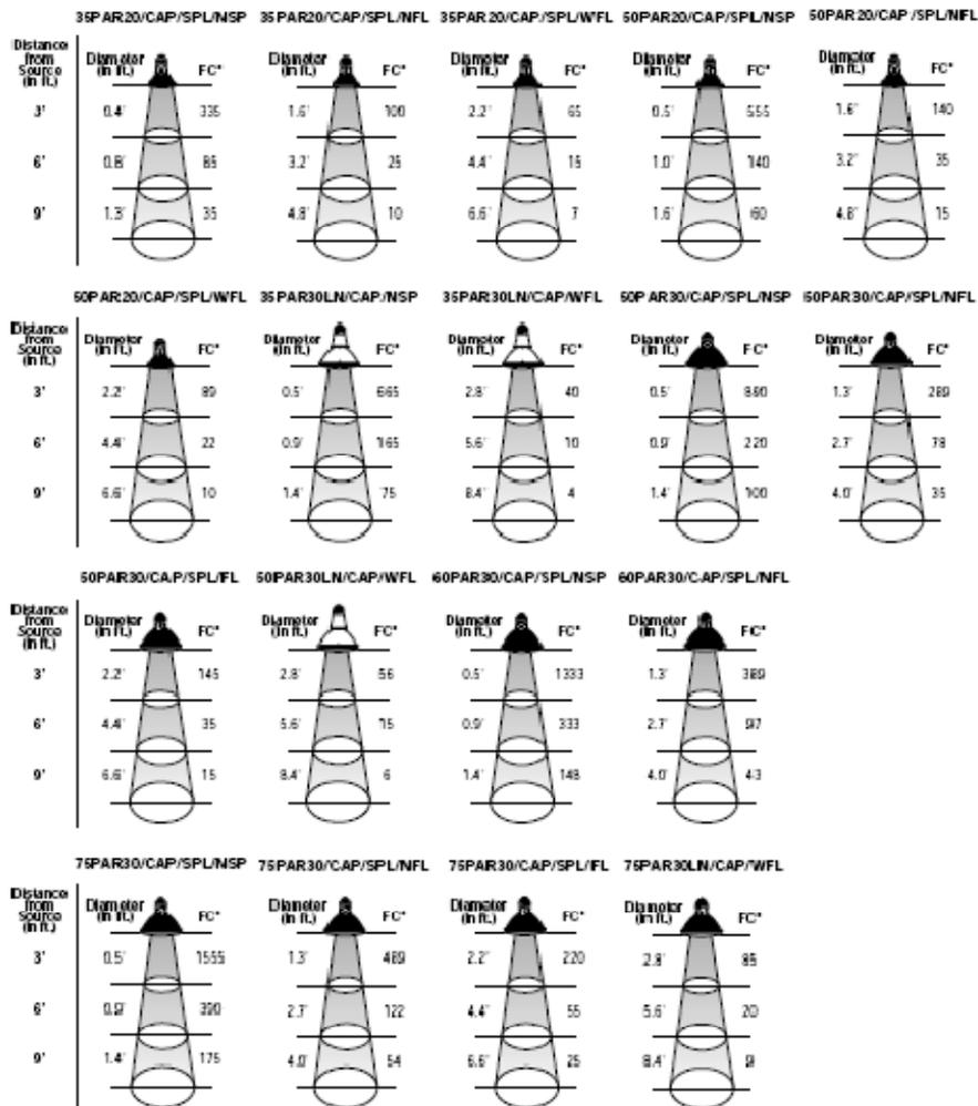
SYLVANIA CAPSYLITE PAR lamps are available in a full range of beam angles to meet the demands of virtually any display or accent lighting application. For each available CAPSYLITE PAR lamp, this table shows how lamp output in footcandles varies as a function of distance.
