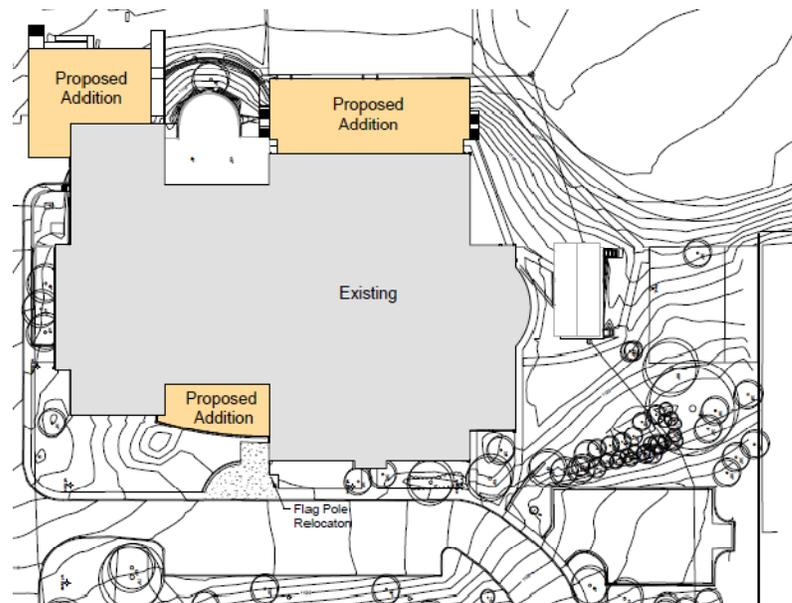
**Figure 5-1 Site Plan of Amanda Arnold Elementary for Proposed Renovations
