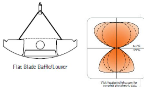
**Figure 3-2: Direct/indirect suspended fixture cross section and light distribution illustration (Focal point).**
