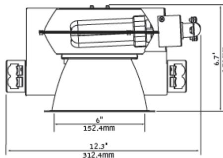
**Figure 3-3: Recessed can light fixture housing and lamp [Focal Point].**
