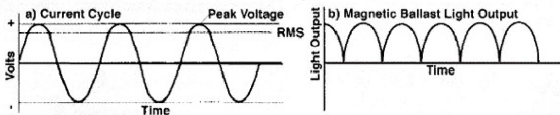
**Figure 2-2: Sinusoidal graph comparing the frequency of current to perceived cycle of light**
