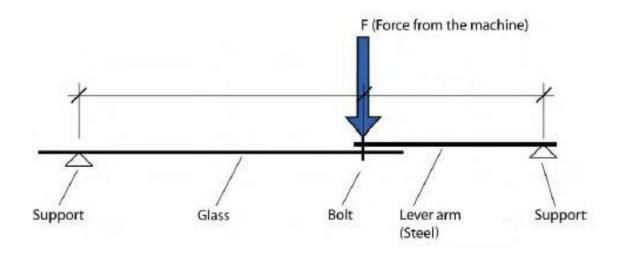
Figure 7-7 Bolt Loaded in Bending (Persson Online)
