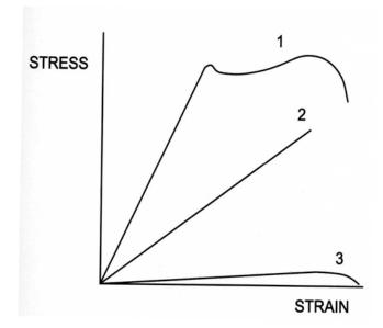
Figure 4-1 Stress-Strain Curve of Common Materials (Loughran 107) 1-Steel 2-Glass 3-Wood
