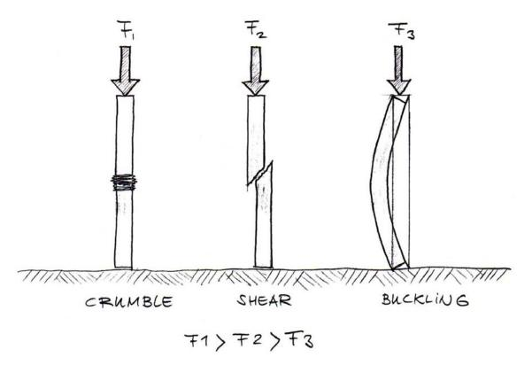
Figure 5-2 Failure Modes of Columns (Nijsse 60)
