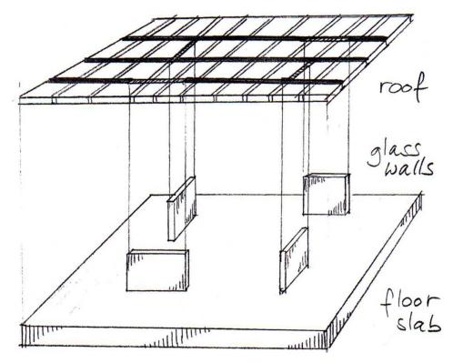
Figure 8-1 Sketch of Structural Glass Wall and Roof Structure (Nijsse 108)
