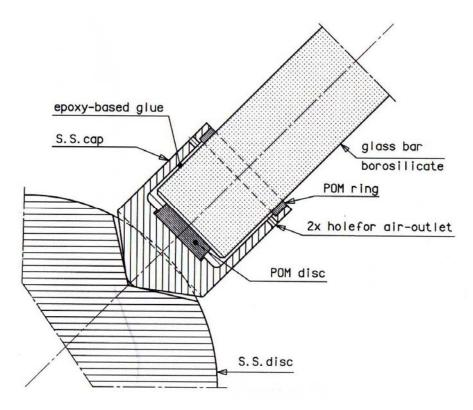
Figure 7-2 Glass Truss Connection (Nijsse 64)
