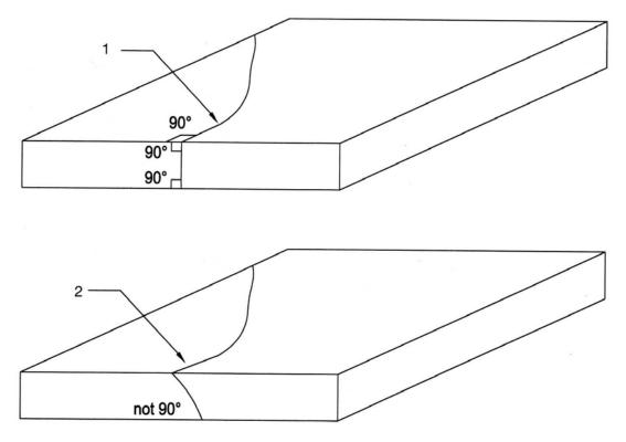
Figure 4-2 Identifying the Cause of Failures (Loughran 26)1 – Thermal break2 – Non-thermal break
