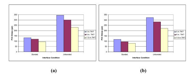
Figure 4.6 PCC Stress vs. Interface Bonding Condition Graph for 7-in. Existing AC Layer and Paved Shoulder (a) AC Modulus 250 ksi and (b) AC Modulus 350 ksi
