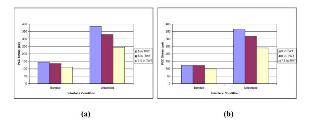
Figure 4.4 PCC Stress vs. Interface Bonding Condition Graph for 5-in. Existing AC Layer and Paved Shoulder (a) AC Modulus 250 ksi and (b) AC Modulus 350 ksi
