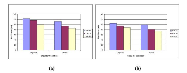
Figure 4.29 PCC Stress vs. Shoulder Condition Graph for 7.5-in. Bonded TWT (a)
