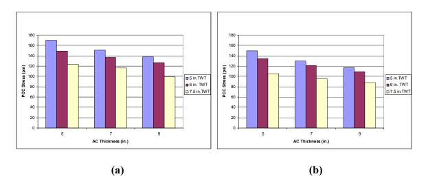
Figure 4.15 PCC Stress vs. Existing AC Thickness Graph for Bonded Condition and
