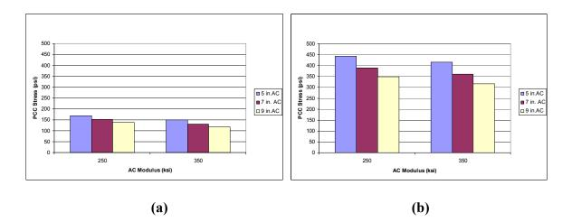
Figure 4.19 PCC Stress vs. Existing AC Modulus Graph for 5-in. TWT and Unpaved
