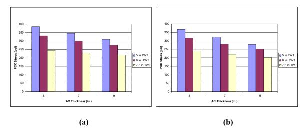
Figure 4.18 PCC Stress vs. Existing AC Thickness Graph for Unbonded Condition and Paved Shoulder (a) AC Modulus 250 ksi and (b) AC Modulus 350 ksi
