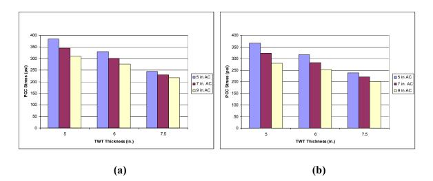
Figure 4.14 PCC Stress vs. TWT Thickness Graph for Unbonded Condition and Paved Shoulder (a) AC Modulus 250 ksi and (b) AC Modulus 350 ksi
