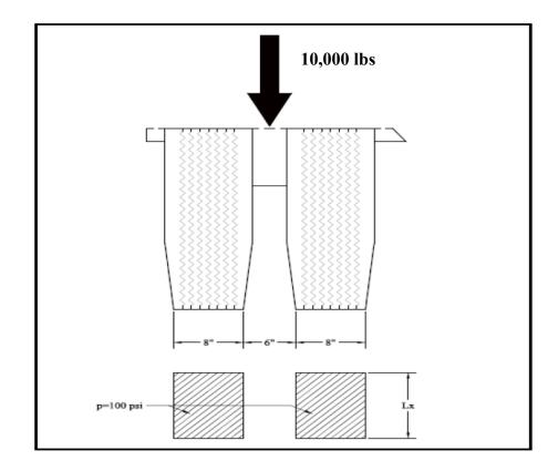
Figure 3.6 Load Model (after Dumitru, 2006)
