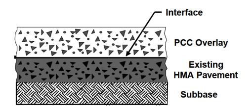
Figure 3.1 Three-Layer Pavement System (McGhee, 1994)
