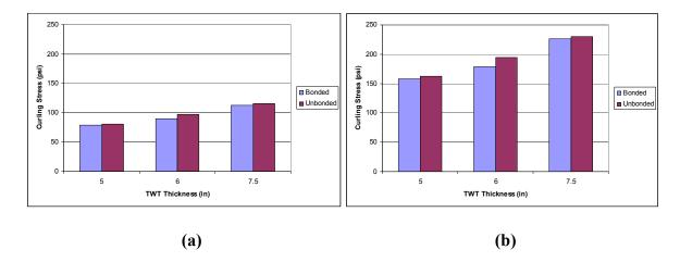
Figure 4.33 PCC Stress vs. TWT Thickness for AC Modulus 350 ksi (a) Temp. Diff. of 1.5<sup>0</sup>F/in and (b) Temp. Diff. 3<sup>0</sup>F/in
