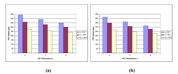
Figure 4.16 PCC Stress vs. Existing AC Thickness Graph for Unbonded Condition and Unpaved Shoulder (a) AC Modulus 250 ksi and (b) AC Modulus 350 ksi
