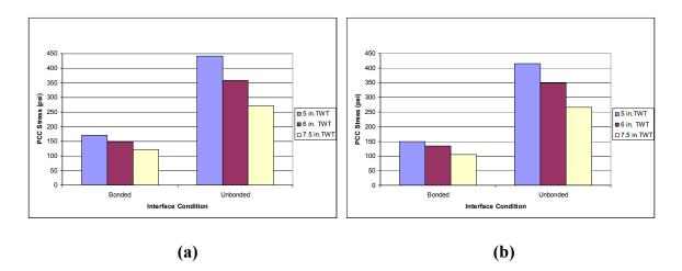
Figure 4.3 PCC Stress vs. Interface Bonding Condition Graph for 5-in. Existing AC Layer and Unpaved Shoulder (a) AC Modulus 250 ksi and (b) AC Modulus 350 ksi
