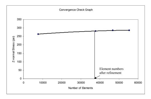
Figure 3.2 Convergence Check Using Z-Normal Stress as a Measure
