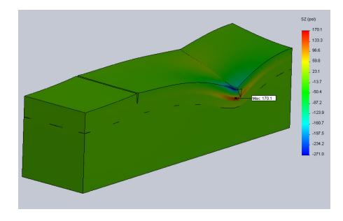
Figure 4.1 Transverse Stress Contour of TWT
