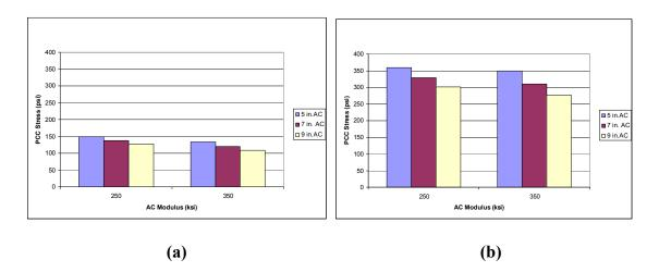
Figure 4.21 PCC Stress vs. Existing AC Modulus Graph for 6-in. TWT and Unpaved
