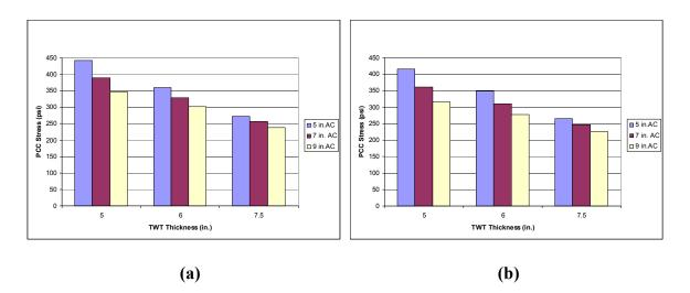
Figure 4.12 PCC Stress vs. TWT Thickness Graph for Unbonded Condition and
