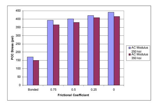
Figure 4.9 PCC Stress vs. Frictional Coefficient Graph for Unpaved TWT
