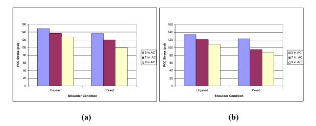
Figure 4.27 PCC Stress vs. Shoulder Condition Graph for 6-in. Bonded TWT (a) AC
