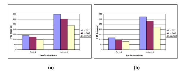
Figure 4.7 PCC Stress vs. Interface Bonding Condition Graph for 9-in. Existing AC Layer and Unpaved Shoulder (a) AC Modulus 250 ksi and (b) AC Modulus 350 ksi
