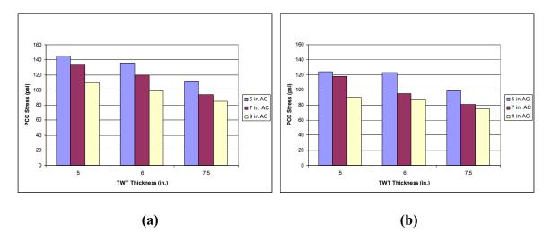
Figure 4.13 PCC Stress vs. TWT Thickness Graph for Bonded Condition and Paved
