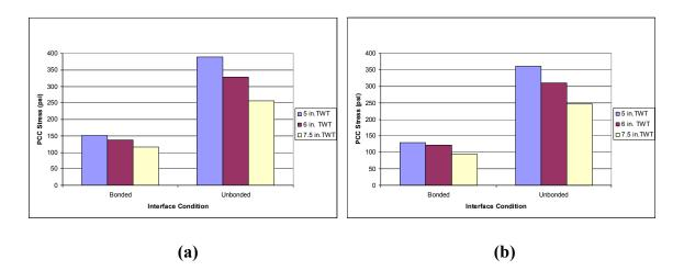
Figure 4.5 PCC Stress vs. Interface Bonding Condition Graph for 7-in. Existing AC Layer and Unpaved Shoulder (a) AC Modulus 250 ksi and (b) AC Modulus 350 ksi
