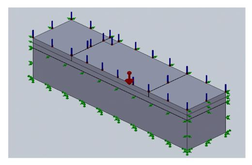
Figure 3.8 Loading Model for Temperature Differential
