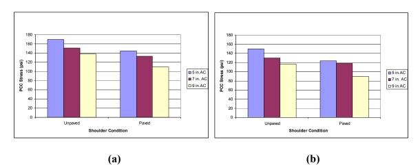
Figure 4.25 PCC Stress vs. Shoulder Condition Graph for 5-in. Bonded TWT (a) AC
