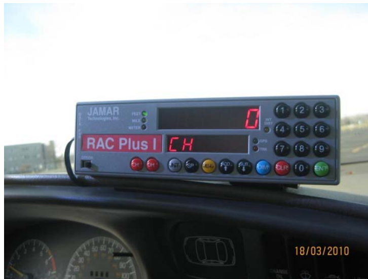
Figure 5.4 Distance measuring instrument measuring distance during the experiment
