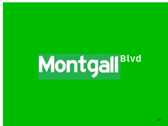
Figure B.3 Sample Slide showing a Street name in Series E-Modified font at 120%
