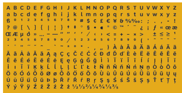
Figure 2.7 Clearview negative contrast font characters for the Series 6-W typeface ( http://clearviewhwy.com/TypefaceDisplay/index.php )
