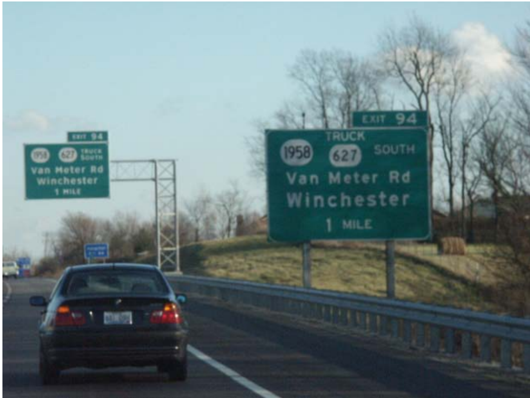
Figure 3.1 A comparison of the old font (right) and the new Clearview font (left) ( http://www.millenniumhwy.net/new_signs_ky_2007/new_signs_ky_2007.html )
