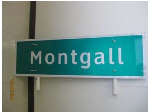
Figure A.1 Montgall Type 4 retro-reflective material and Clearview 5 –W font
