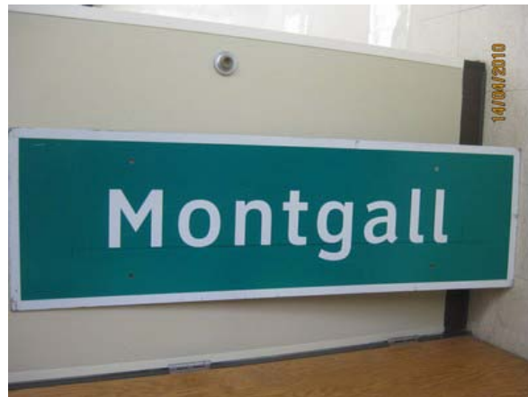
Figure A.8 Montgall in Type 1 retro-reflective material and Clearview 5-W-R font
