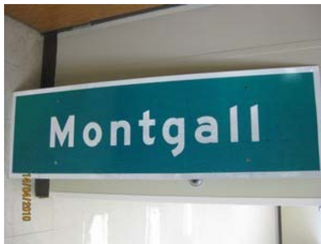
Figure A.2 Montgall DG3 retro-reflective material and Series E-Modified font
