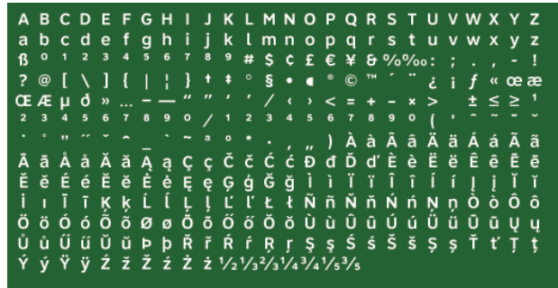
Figure 2.5 Clearview positive contrast font characters for the Series 6-W typeface ( http://clearviewhwy.com/TypefaceDisplay/index.php )
