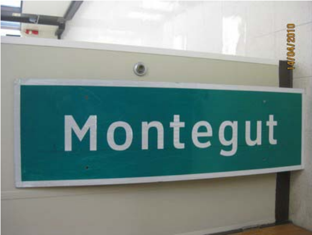
Figure A.9 Montegut in Type 4 retro-reflective material and Clearview 5-W-R font
