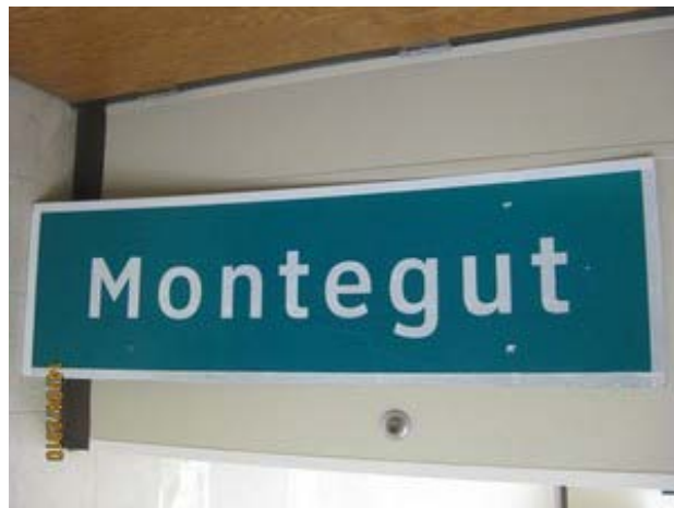
Figure A.4 Montegut in DG3 retro-reflective sheeting material and Clearview 5-W font
