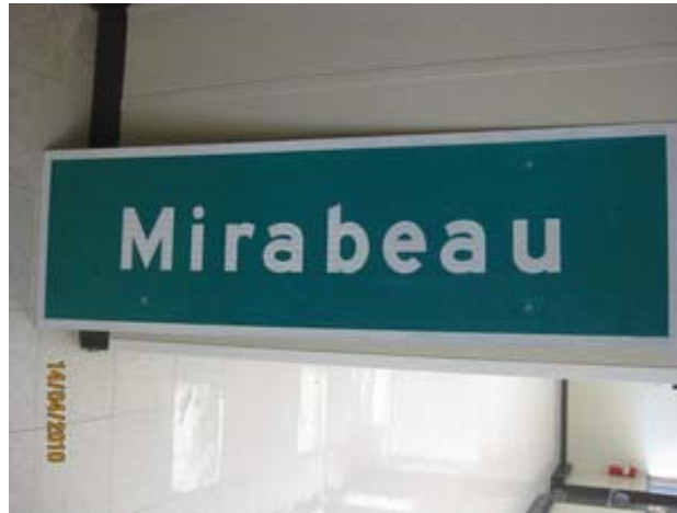
Figure A.3 Mirabeau in Type 4 retro-reflective material and Series E-Modified font
