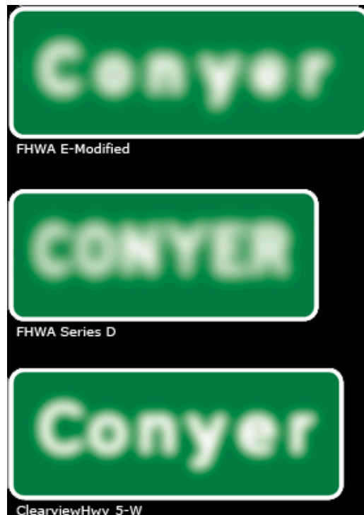
Figure 2.2 Halation phenomenon observed in different font types
