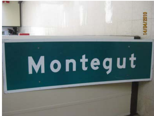
Figure A.6 Montegut in Type 1 retro-reflective material and Series E-Modified font
