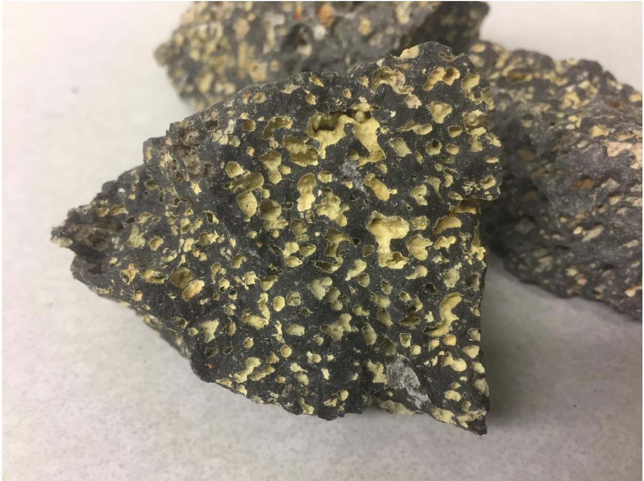
Figure 3.5 Discarded sample Nabesna 9 displays bright yellow material lining the vesicles, suggesting heavy secondary alteration.
