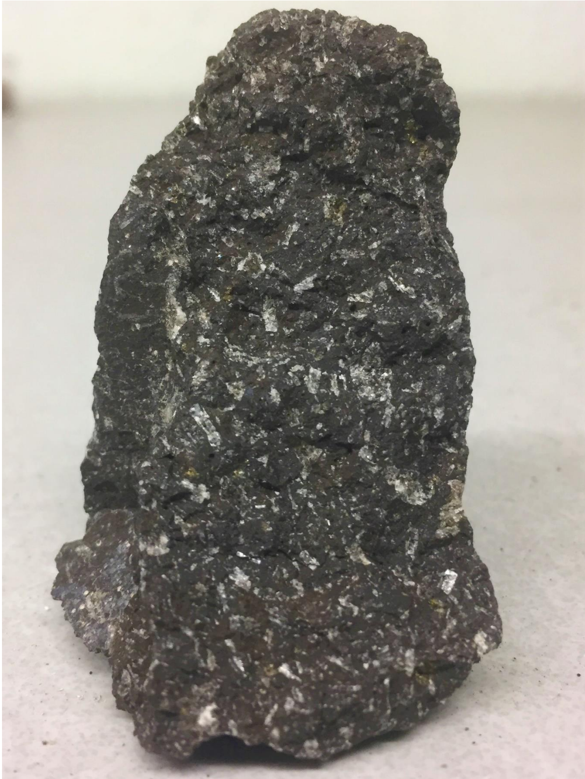
Figure 3.6 Sanford 6, an example of a mafic rock with porphyritic-volcanic texture from the dataset.
