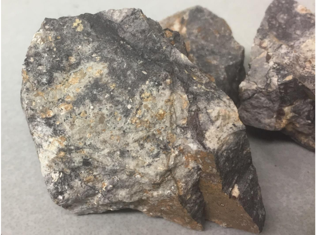
Figure 3.4 Discarded sample Cross 8 displays pervasive groundmass and primary mineral alteration/replacement.
