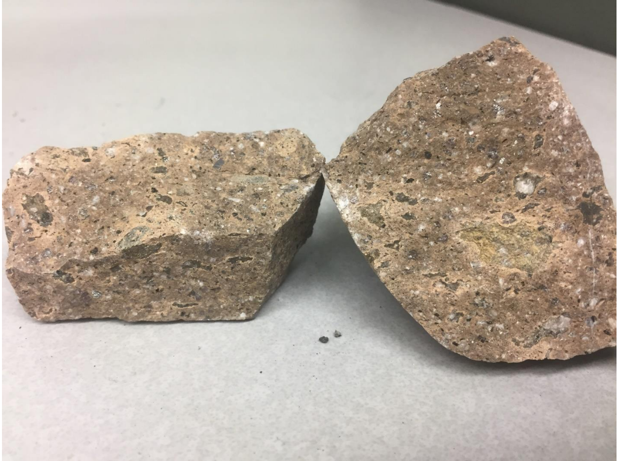
Figure 3.11 Chisana 6, another example of a rock with pyroclastic texture from our dataset.
