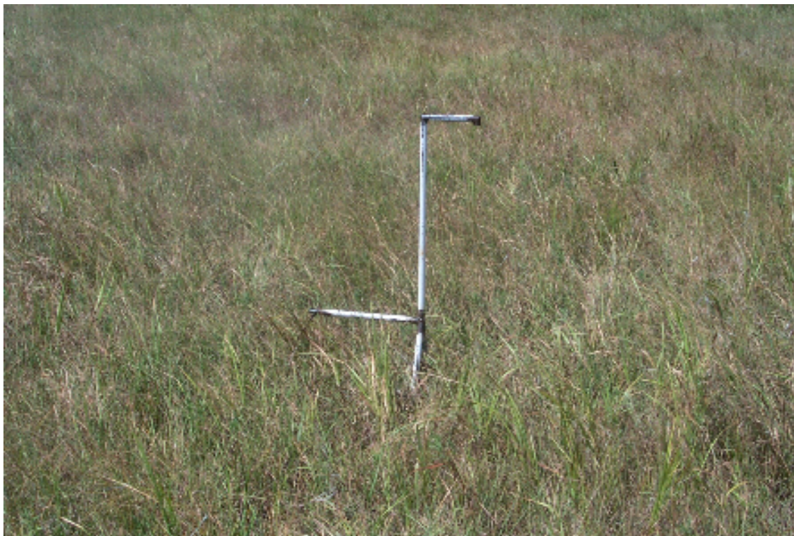
Figure E.2 Modified step-point frame used in botanical composition collections
