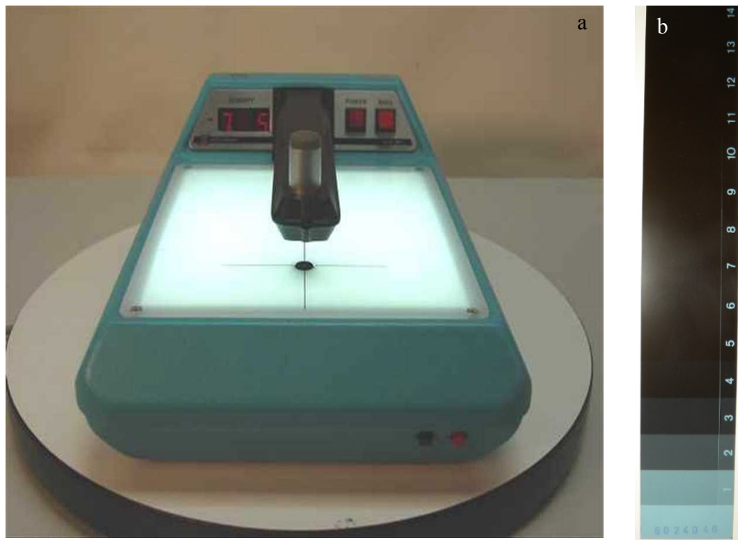
Figure 4-26. X-RITE 301 densitometer used to measure the optical density (a), calibrated transmission set (b).
