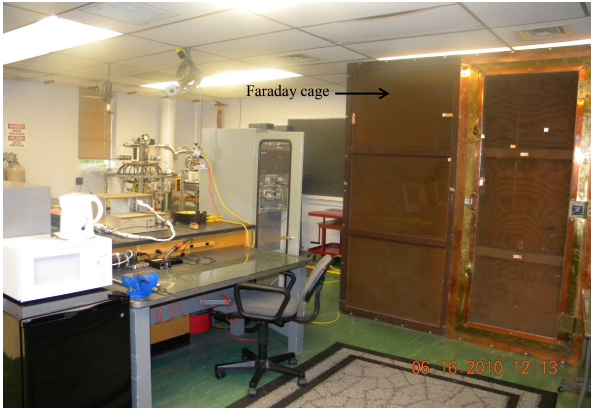
Figure 3-24. The Faraday cage that contains the oscilloscopes.
