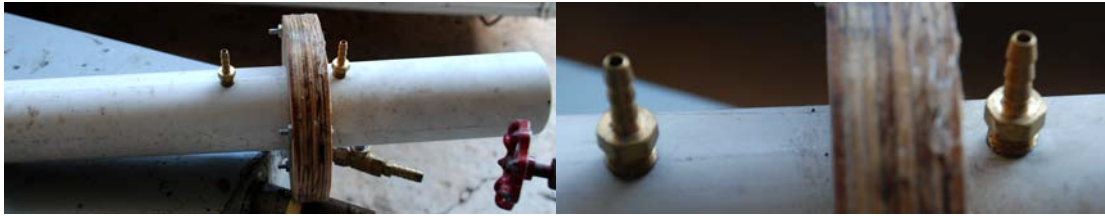
Figure 3.12 Actual flow nozzle installation
