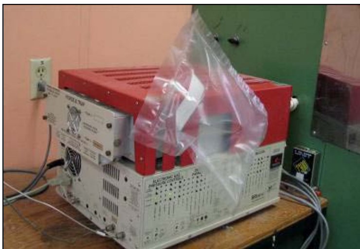
Figure 4.3 Syngas composition analysis using a SRI 8610s GC
