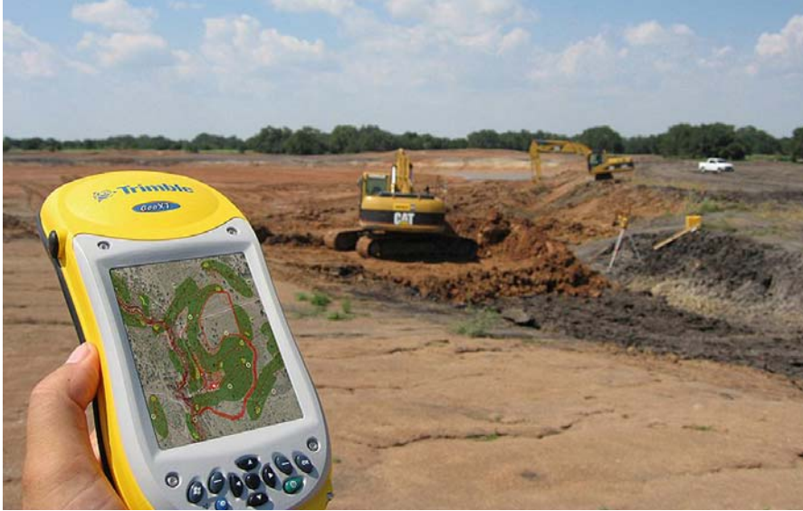
Figure 2.22 – Use of GPS Hand-Held Unit During Construction at Wolf Point Club, Port Lavaca, Texas (mnuzzo.com)
