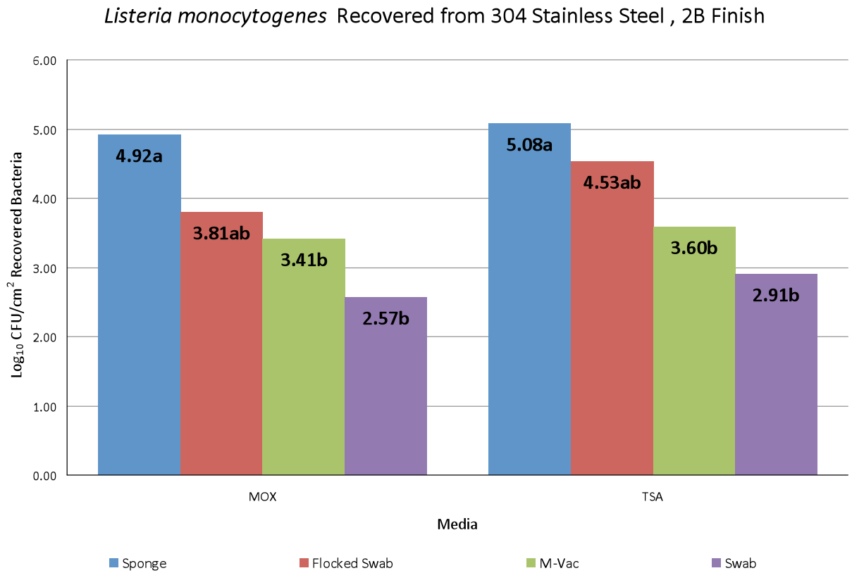
Figure 3.5 Listeria monocytogenes Sampled from 304 Stainless Steel with a 2B Finish.
